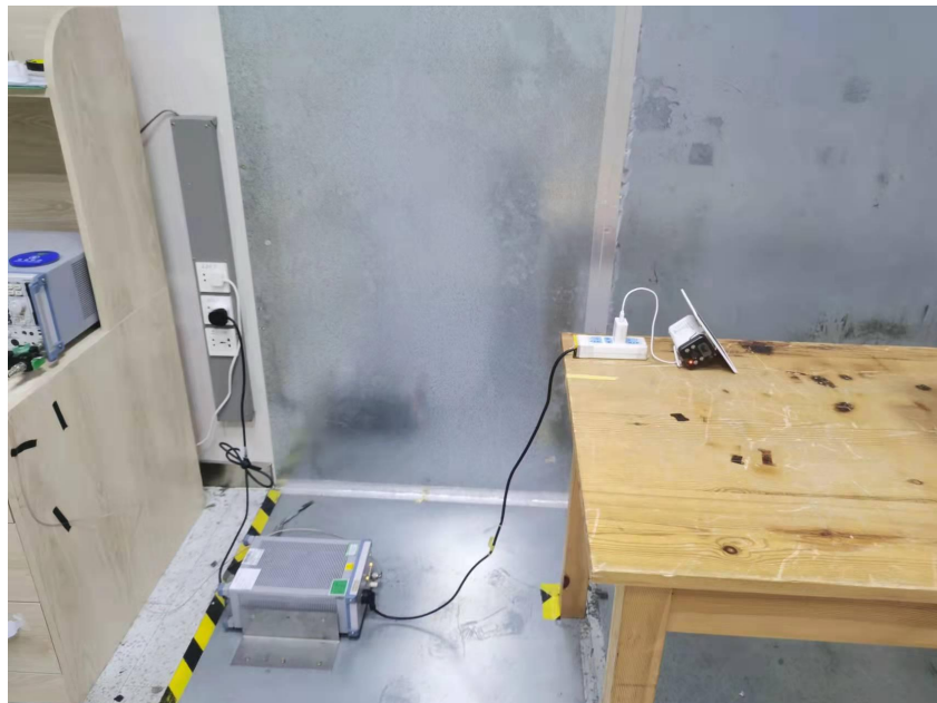
Radiated Spurious Emissions From 30MHz-1000MHz
