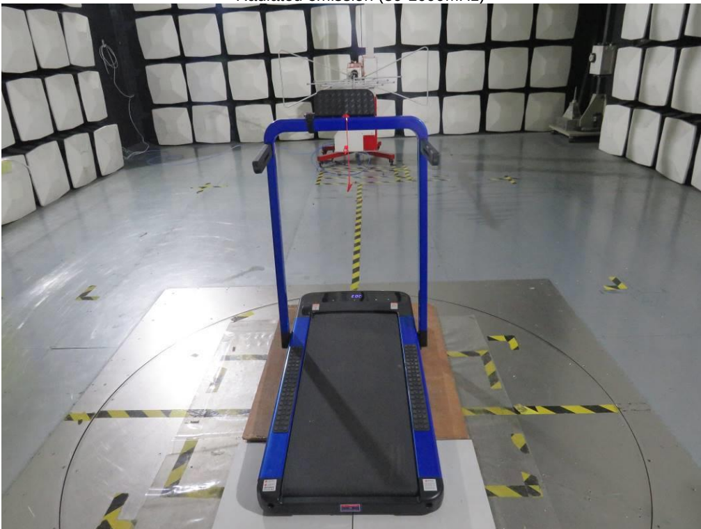
Radiated emission (30-1000MHz)
