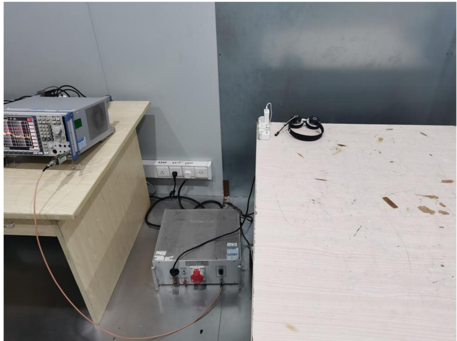
Conducted Emission Test Setup
