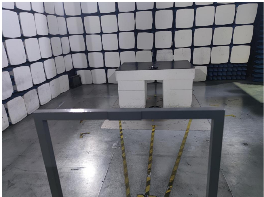
Radiation Emission Test Setup (Below 30MHz)
