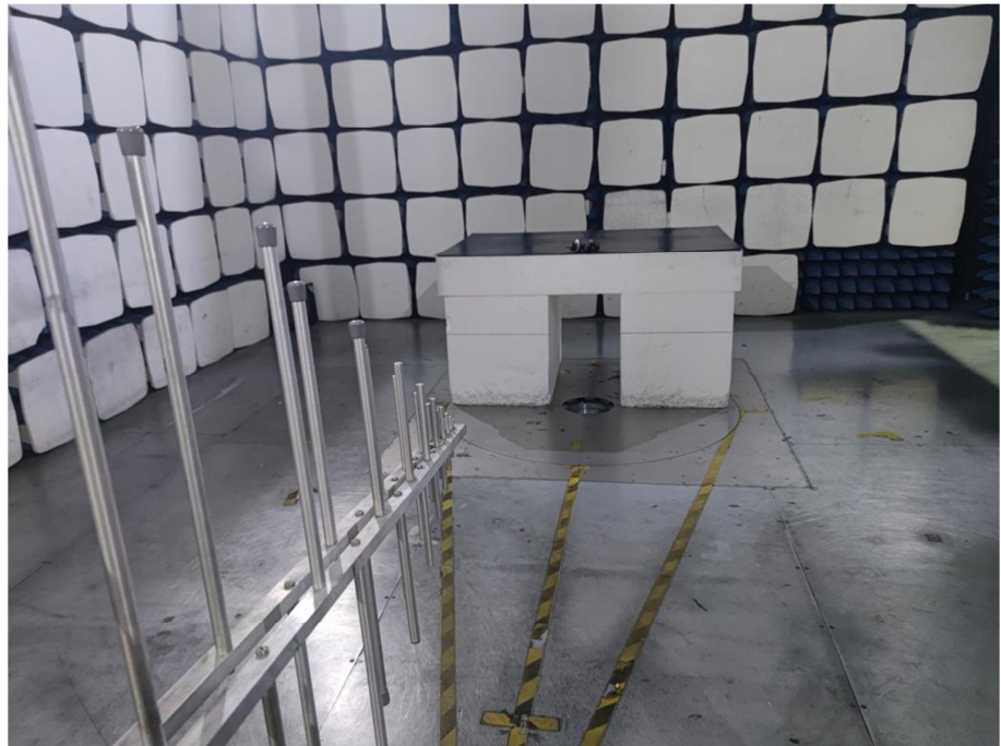
Radiation Emission Test Setup (30MHz to 1GHz)
