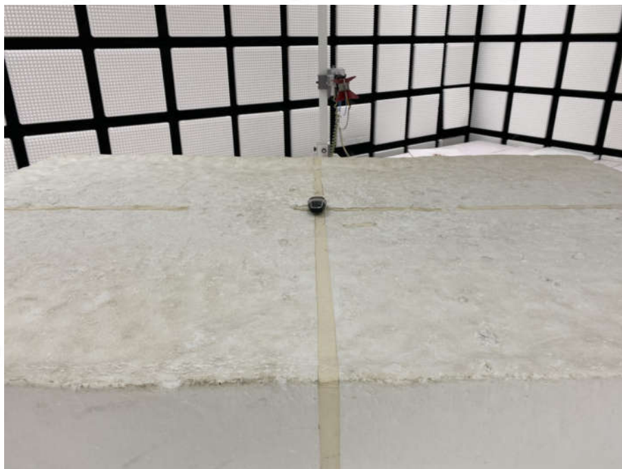
Radiated spurious emission Test Setup-3(Above 1GHz)
