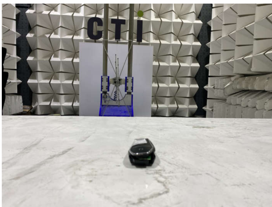
Radiated emission Test Setup-4(30MHz~1GHz)close up photo
