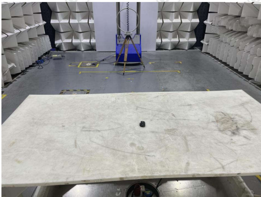
Radiated emission Test Setup-1(9kHz~30MHz)
