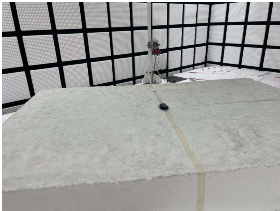
Radiated spurious emission Test Setup-3(Above 1GHz)
