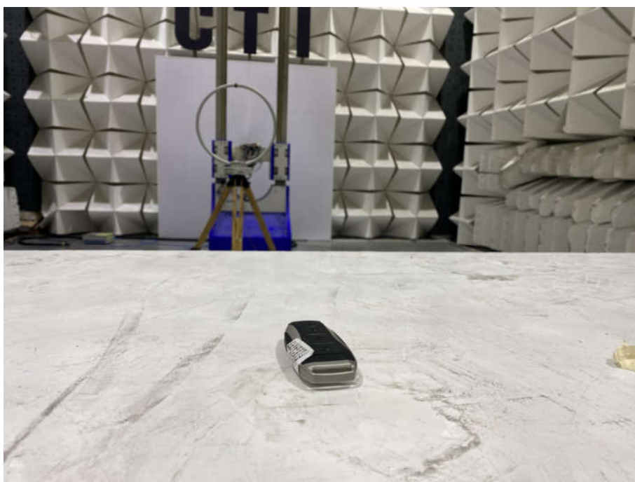
Radiated emission Test Setup-2(9kHz~30MHz)close up photo
