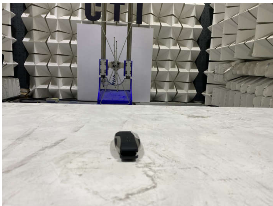
Radiated emission Test Setup-4 (30MHz~1GHz)close up photo
