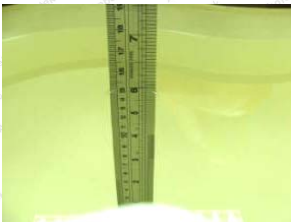
Photo of Liquid Height for Head SAR
