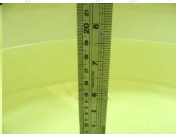
Photo of Liquid Height for Body SAR
