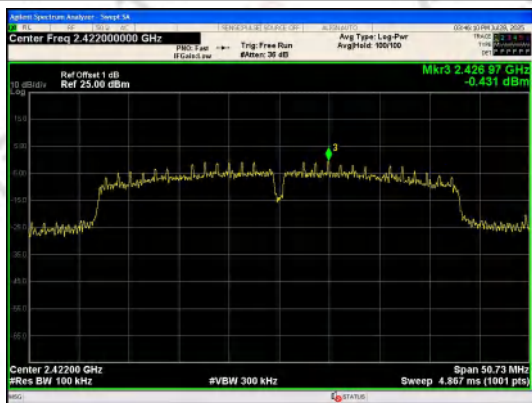
In-Band Reference Level IEEE 802.11n_Channel 3_40MHz_Antenna 0
