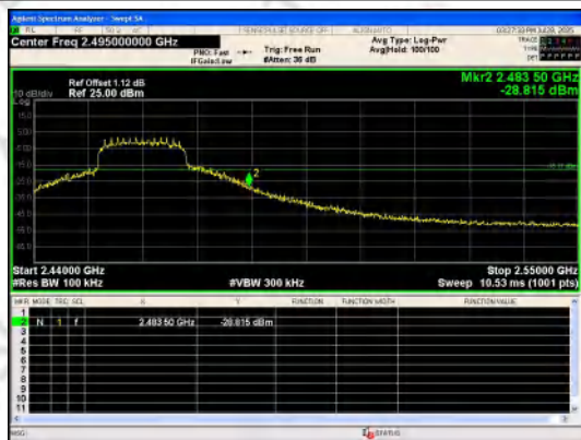
Out Of Band Emission IEEE 802.11g_Channel 11_20MHz_Antenna 0
