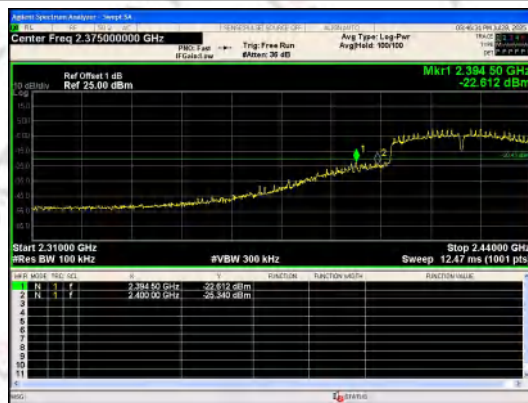
Out Of Band Emission IEEE 802.11n_Channel 3_40MHz_Antenna 0
