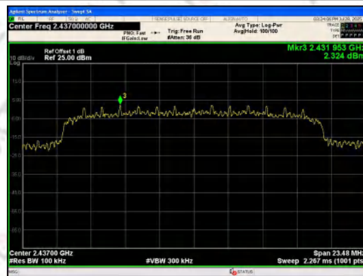
In-Band Reference Level IEEE 802.11g_Channel 6_20MHz_Antenna 0
