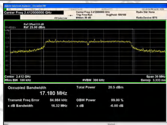
IEEE 802.11g_Channel 1_20MHz_Antenna 0
