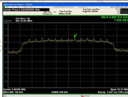
In-Band Reference Level IEEE 802.11g_Channel 11_20MHz_Antenna 0
