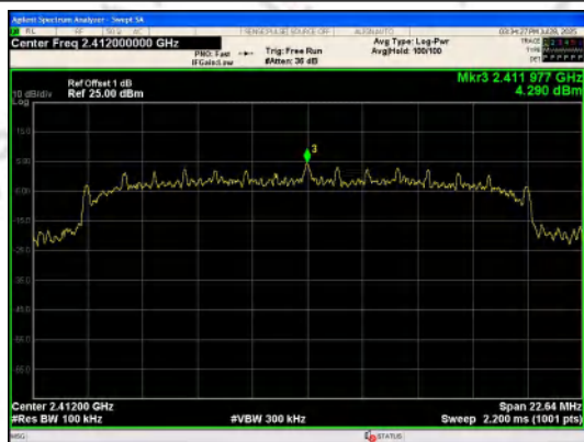
Out Of Band Emission IEEE 802.11g_Channel 11_20MHz_Antenna 0
