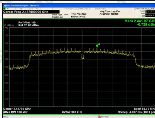
In-Band Reference Level IEEE 802.11n_Channel 6_40MHz_Antenna 0
