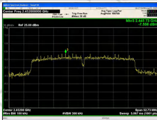
In-Band Reference Level IEEE 802.11n_Channel 9_40MHz_Antenna 0
