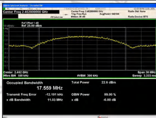
IEEE 802.11b_Channel 11_20MHz_Antenna 0
