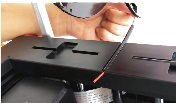
7. Insert the filament into the filament guide.
