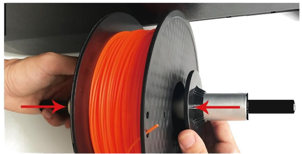
4. Put the gasket left and right to fix the filament.
