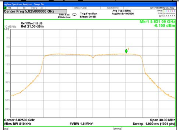
W58_11n20_Higher_Power Spectrum Density
