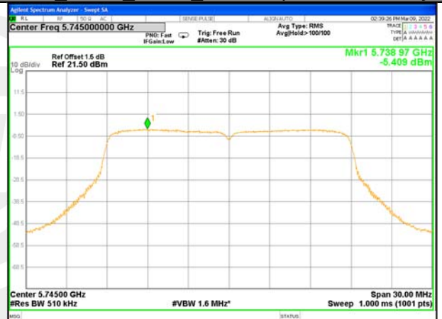
W58_11n20_Higher_Power Spectrum Density
