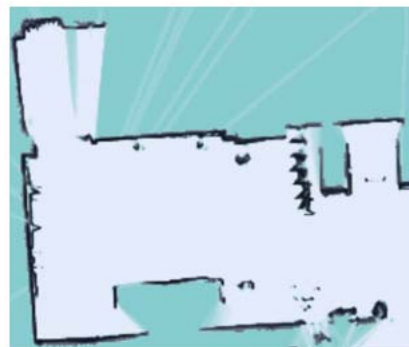
The map scanned by the robot's laser
