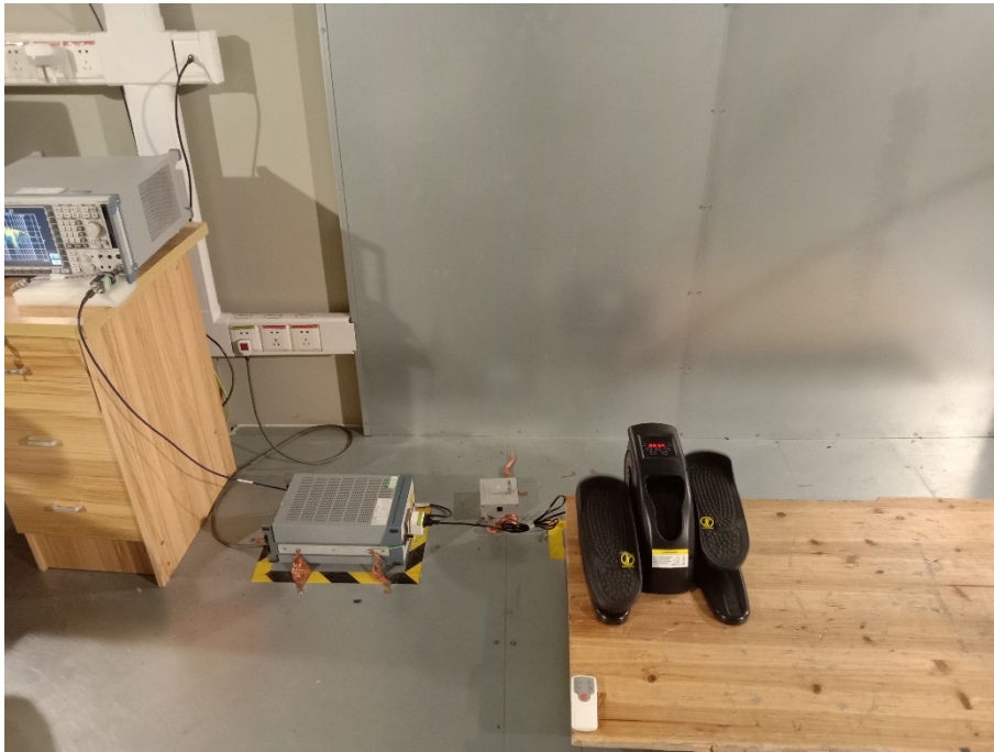
Photograph of test setup for Conducted Emission
