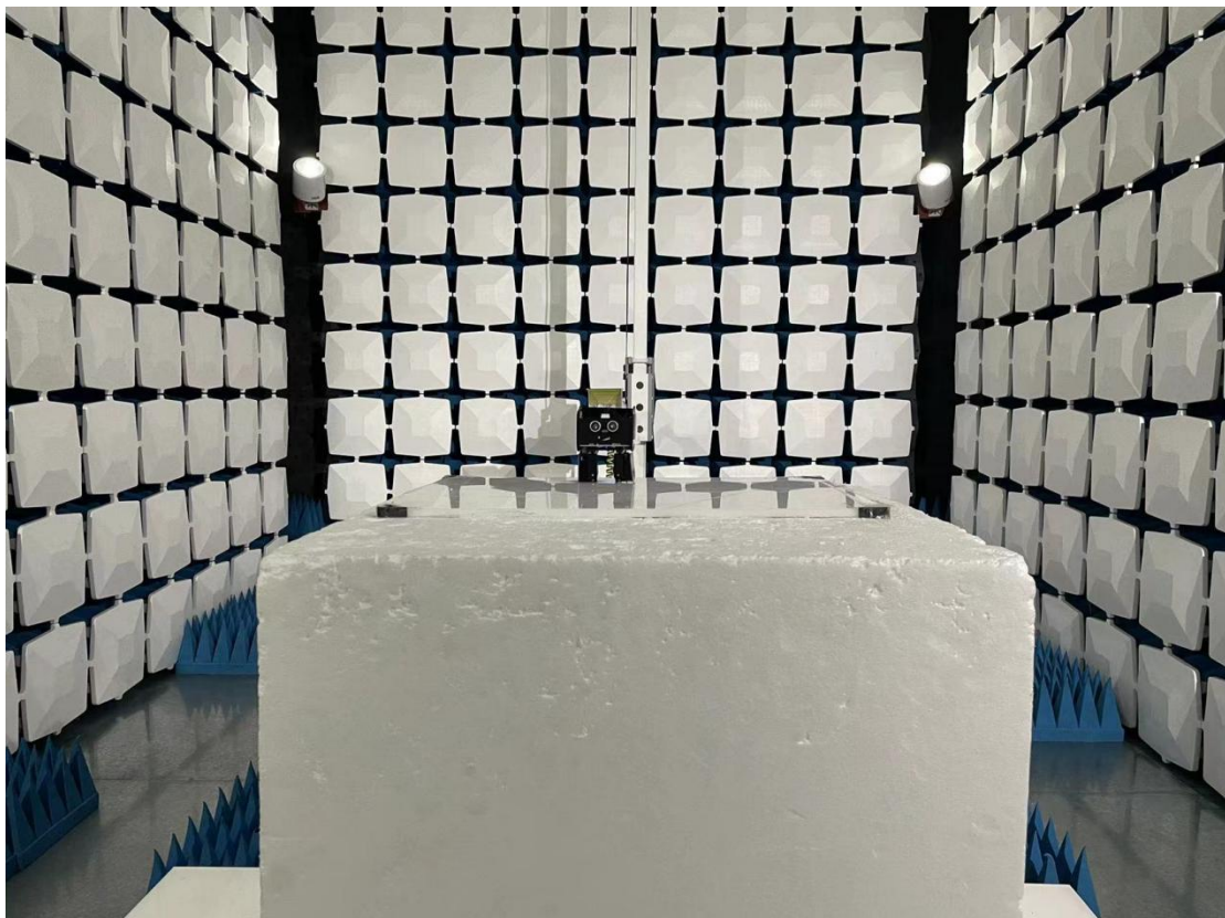
Above 1GHz for radiated emission test setup
