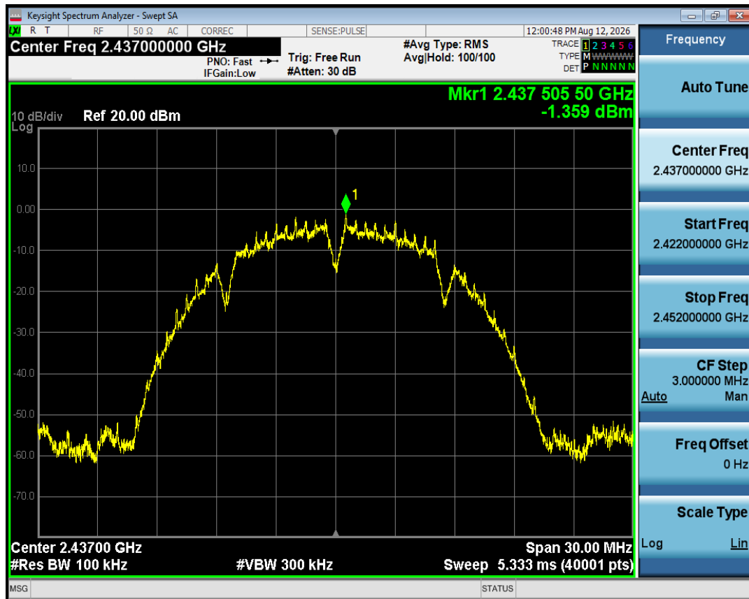
Tx. Spurious NVNT b 2437MHz Ant1 Ref
