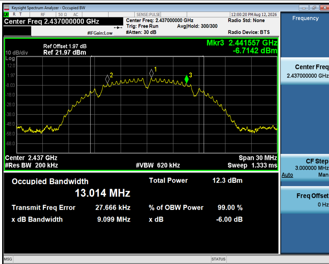
-6dB Bandwidth NVNT b 2437MHz Ant1
