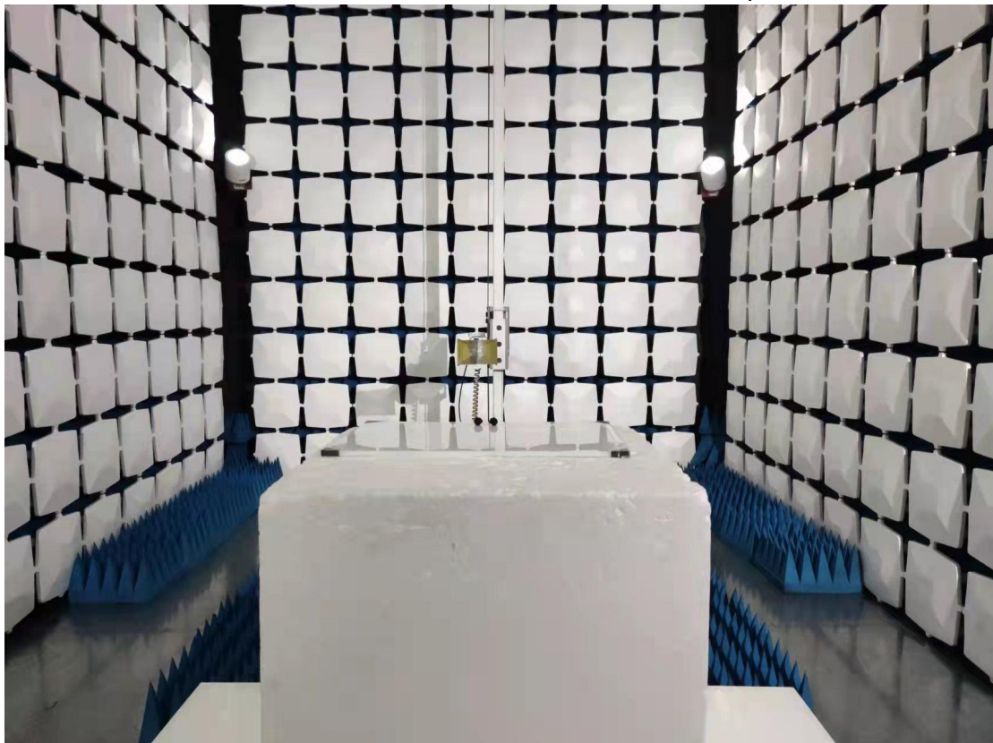
Above 1GHz for radiated emission test setup
