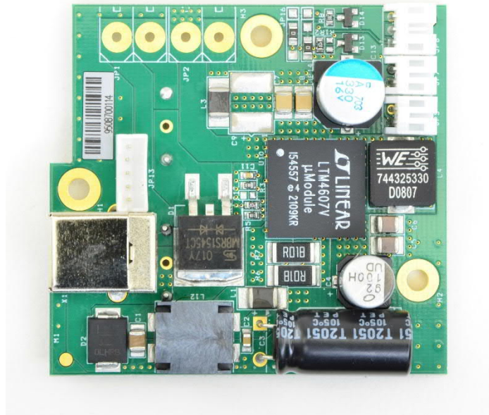
EUT_PCB DC-DC converter front side view (Photos provided by the applicant)
