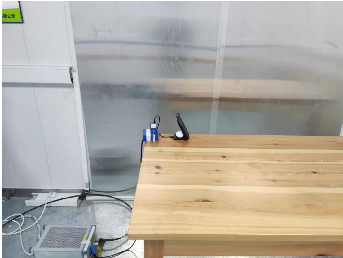
Conducted emission test setup
