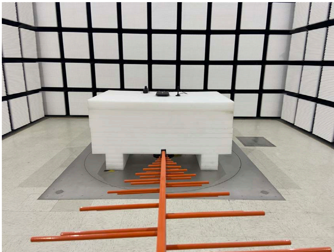
Radiated Emission Above 1GHz View
