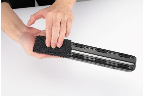
Figure 3- 1 Clean The CIS
