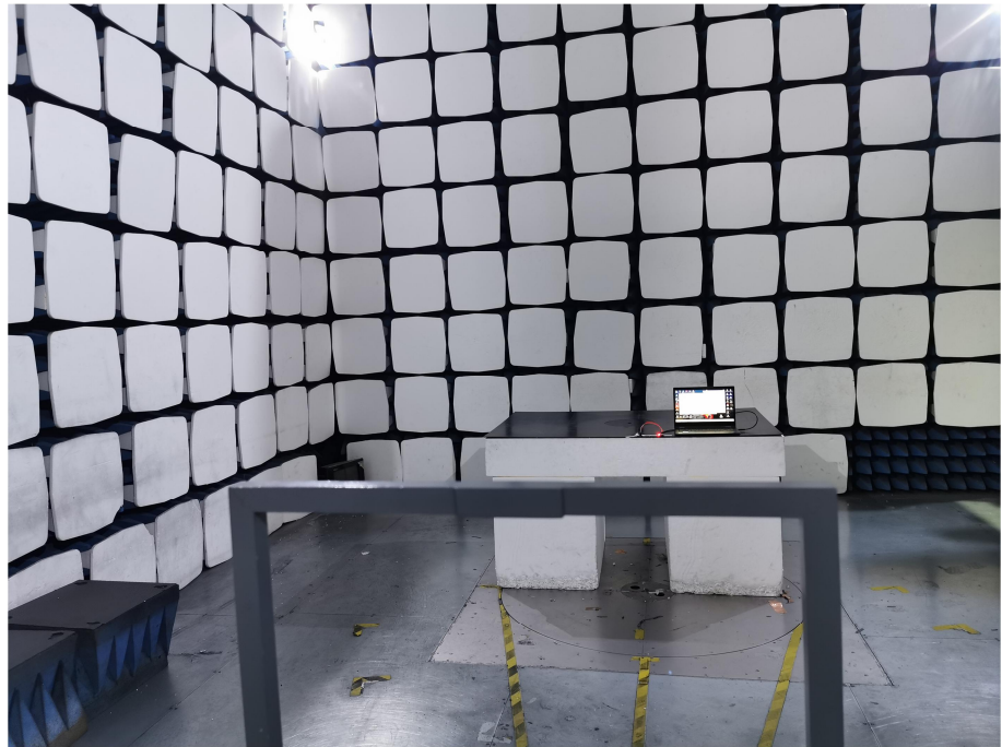
Radiation Emission Test Setup (Below 30MHz)
