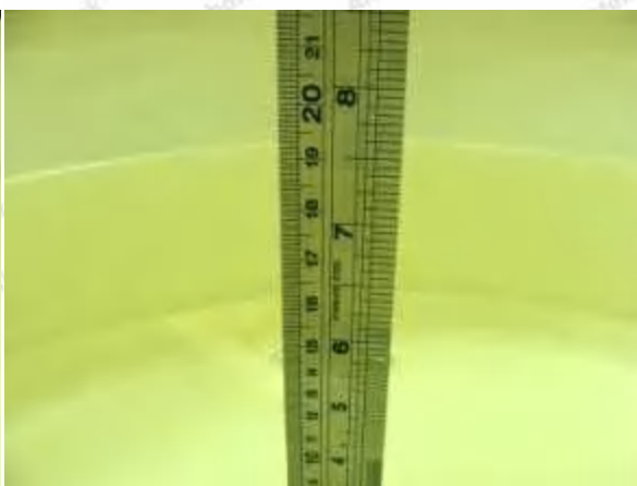
Photo of Liquid Height for Body SAR
