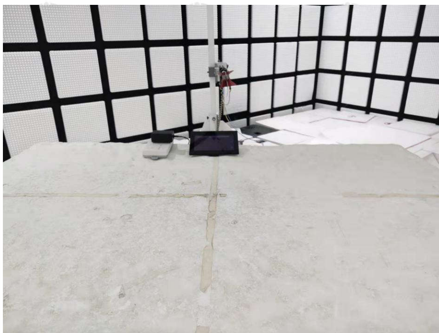
Radiated spurious emission Test Setup-2(Above 1GHz)
