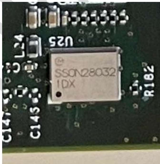
Figure 3 - Wi-Fi/Bluetooth module (detail)
