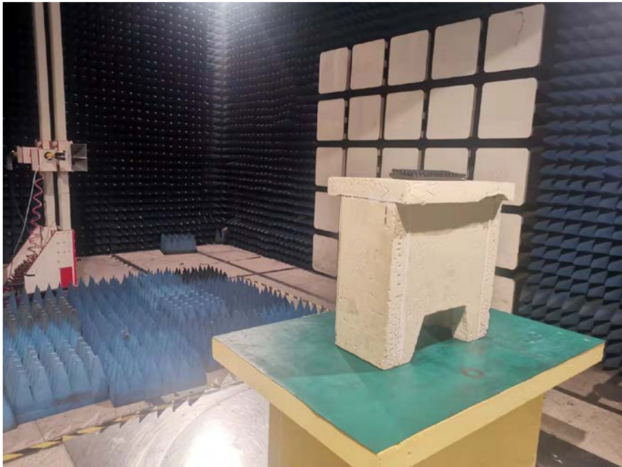
Spurious Emission Test Setup (Above 1GHz)
