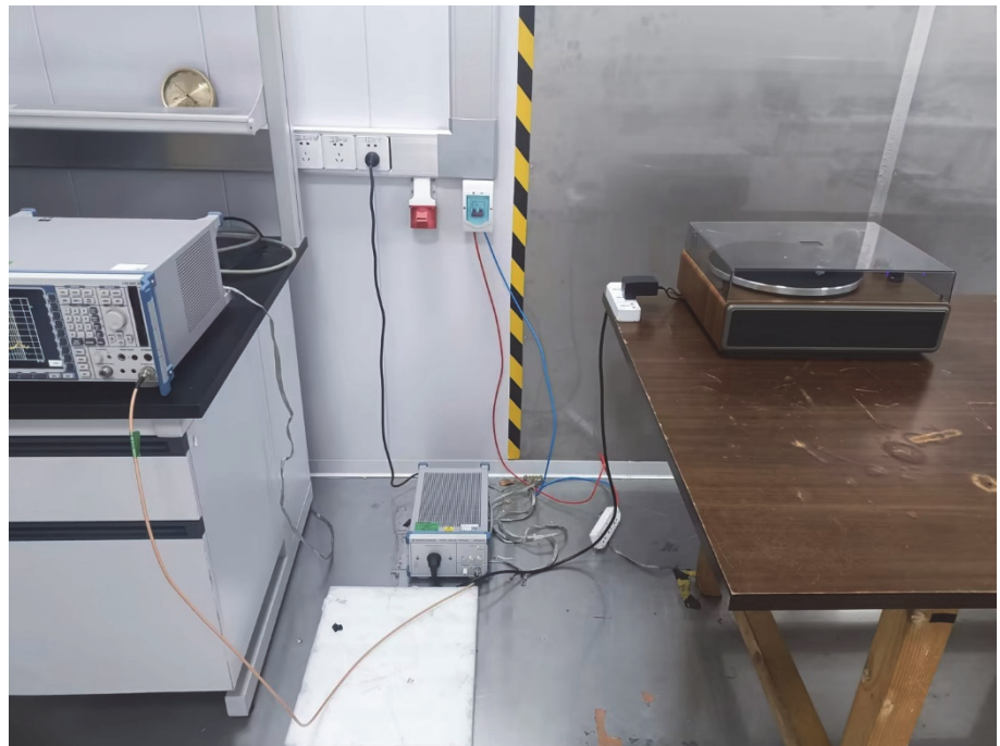
Conducted Emission Test Setup
