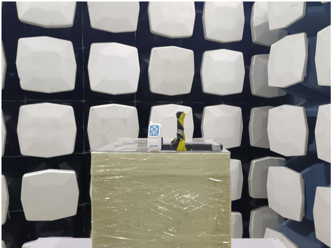
18GHz to 40GHz (The EUT placed at the center of the turntable)
