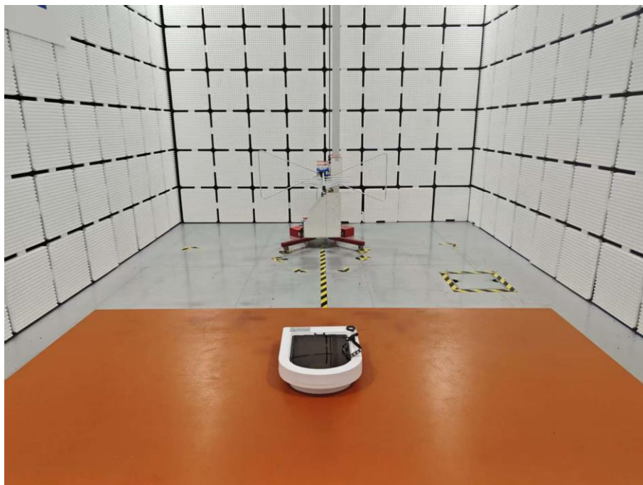
Radiated Emission Above 30MHz
