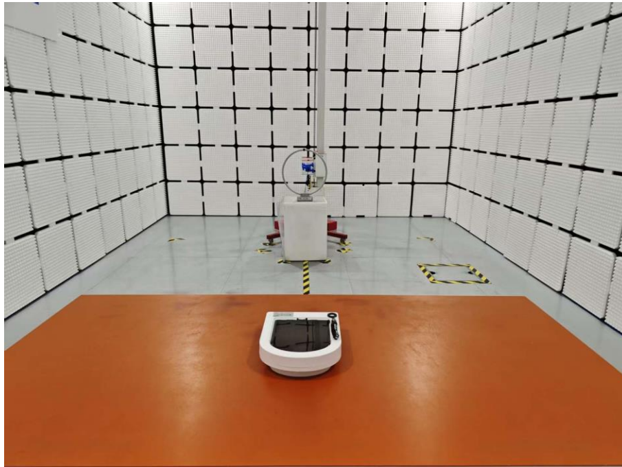
Radiated Emission Above 30MHz
