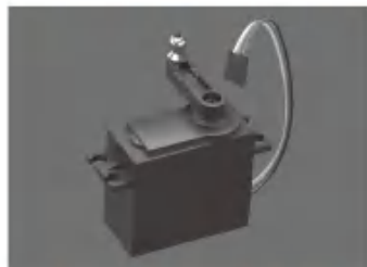
STEERING SERVO (3-WIRE, 6KG)
