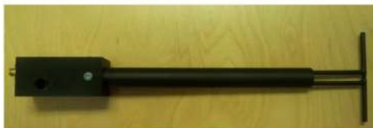
Figure 1 – MVG COMOSAR Validation Dipole
