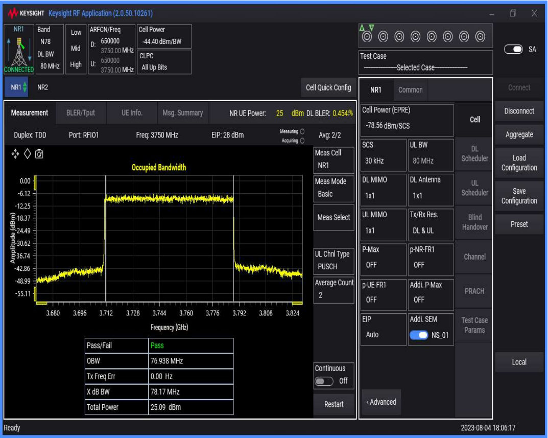
n78(3700-3800) SCS=30kHz DFT_QAM64 BW=90MHz Channel=650000 RB=240@0
