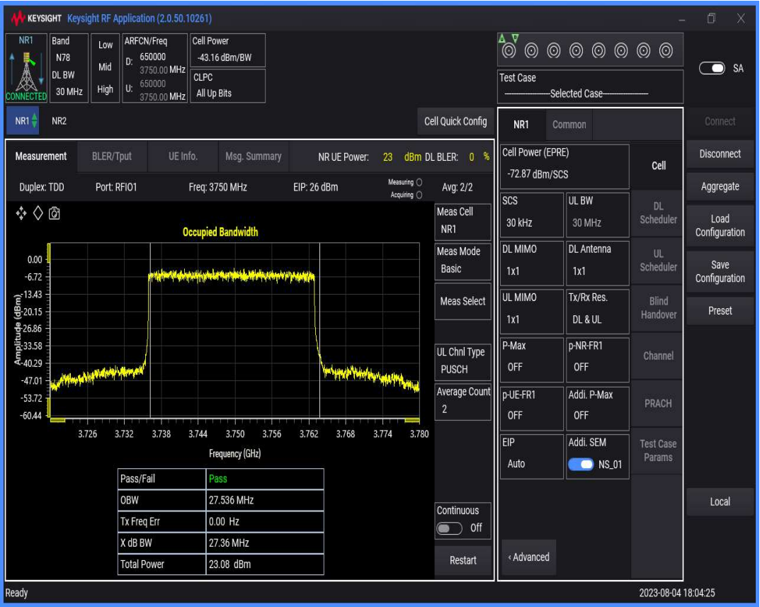
n78(3700-3800) SCS=30kHz DFT_QAM256 BW=40MHz Channel=650000 RB=100@0
