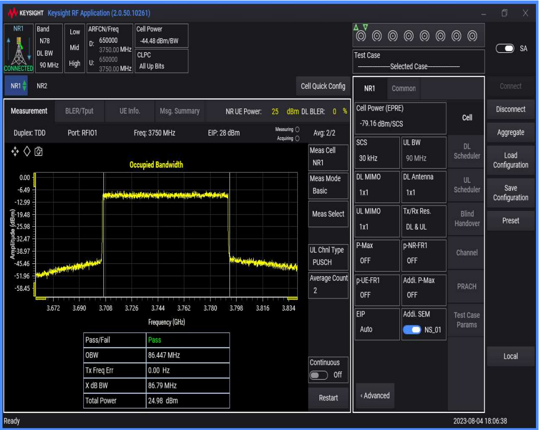
n78(3700-3800) SCS=30kHz DFT_QAM256 BW=100MHz Channel=650000 RB=270@0
