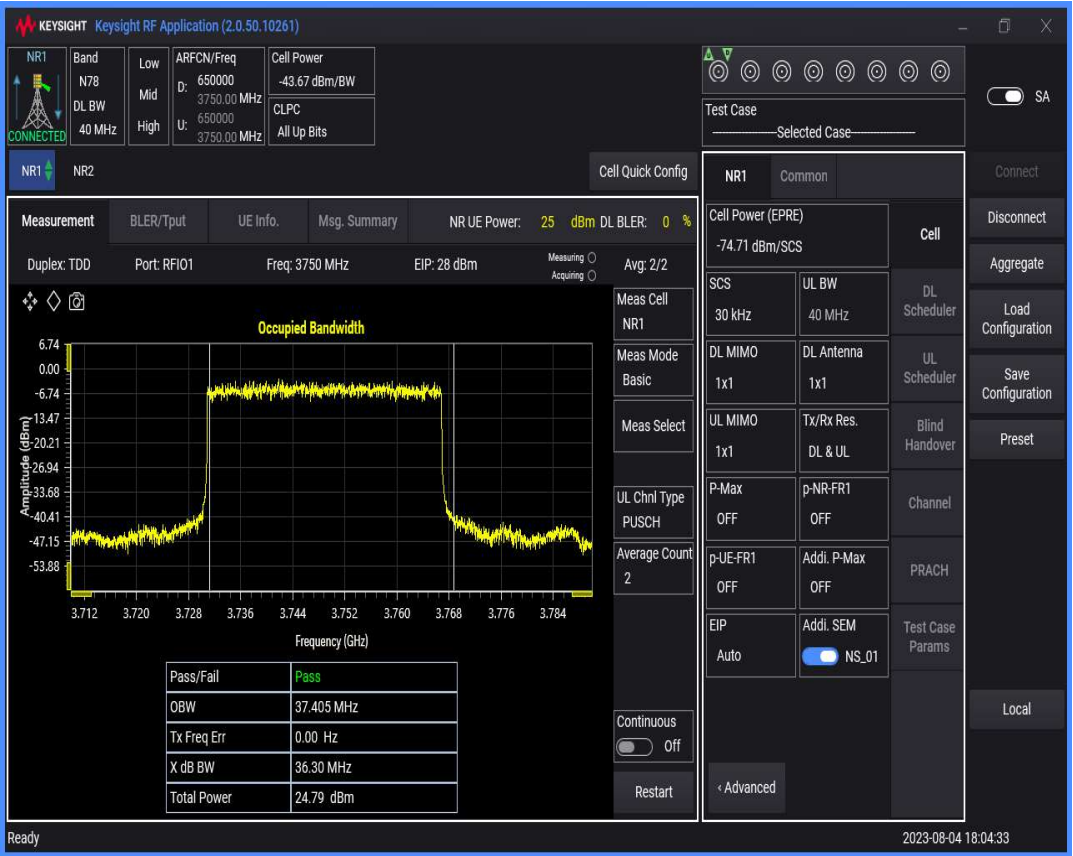
n78(3700-3800) SCS=30kHz DFT_BPSK BW=50MHz Channel=650000 RB=128@0
