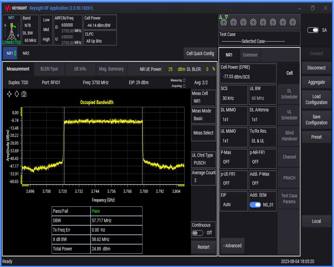
n78(3700-3800) SCS=30kHz DFT_BPSK BW=70MHz Channel=650000 RB=
