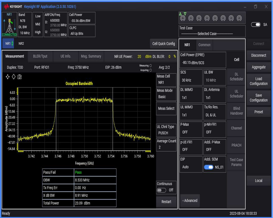
n78(3700-3800) SCS=30kHz DFT_QAM256 BW=15MHz Channel=650000 RB=36@0
