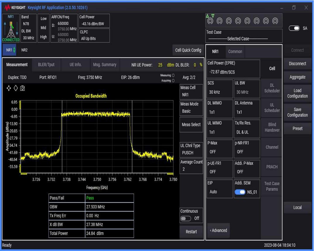
n78(3700-3800) SCS=30kHz DFT_BPSK BW=40MHz Channel=650000 RB=100@0
