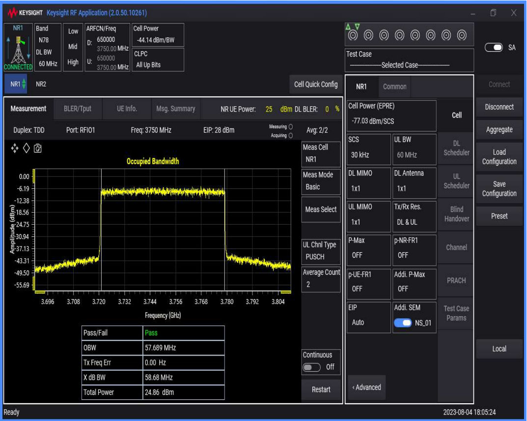
n78(3700-3800) SCS=30kHz DFT_QPSK BW=70MHz Channel=650000 RB=
