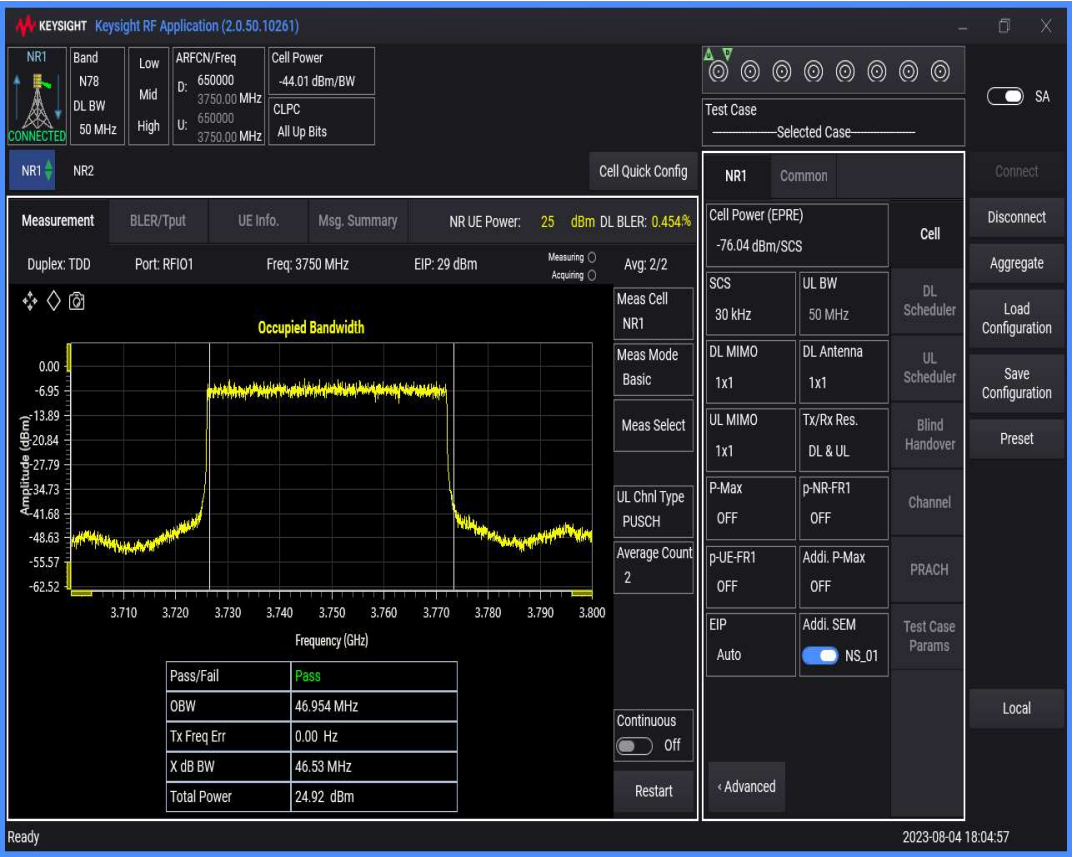
n78(3700-3800) SCS=30kHz DFT_BPSK BW=60MHz Channel=650000 RB=162@0
