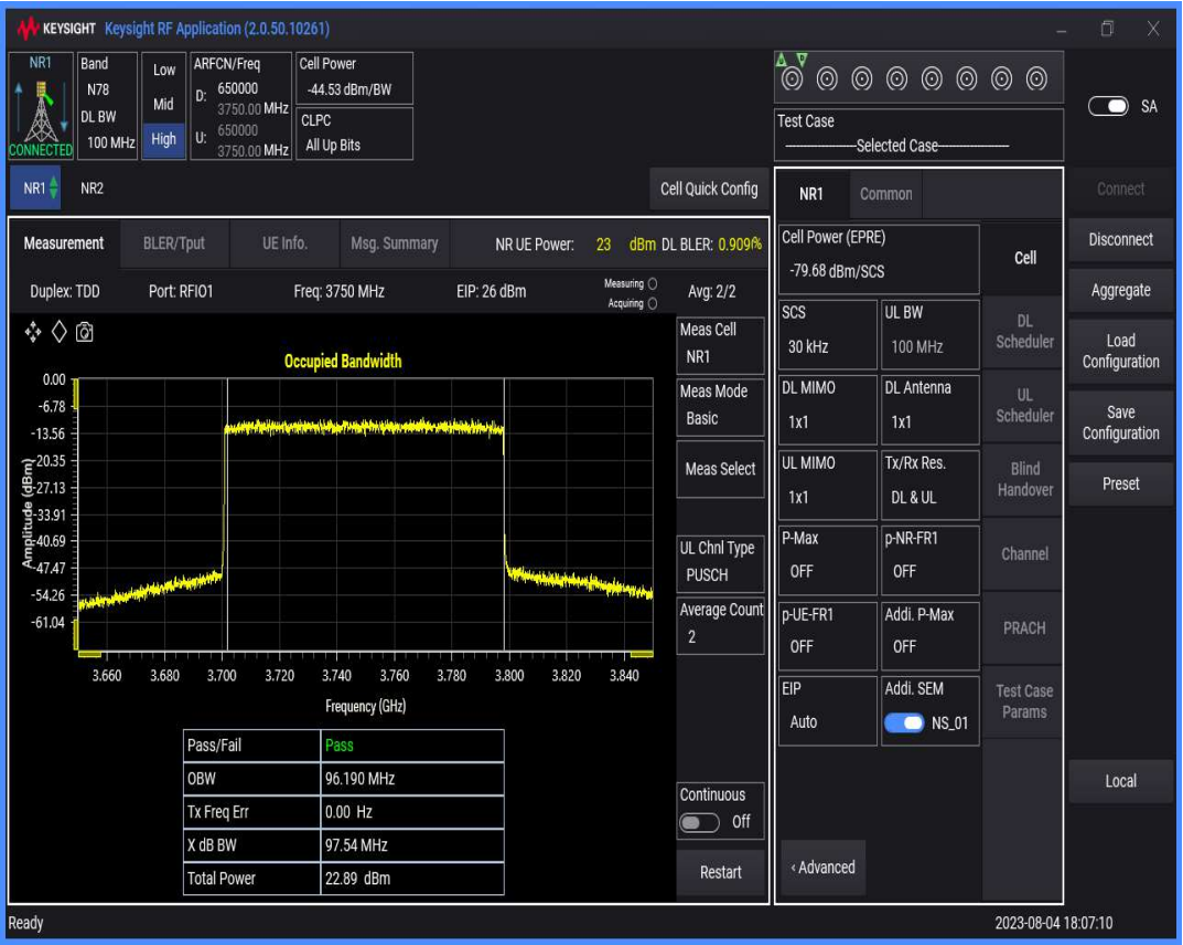
n78(3700-3800) SCS=30kHz DFT_QAM256 BW=10MHz Channel=650000 RB=24@0
