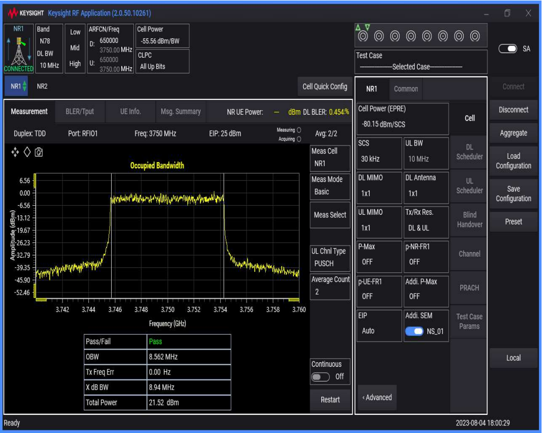
n78(3700-3800) SCS=30kHz DFT_QAM64 BW=15MHz Channel=650000 RB=36@0
