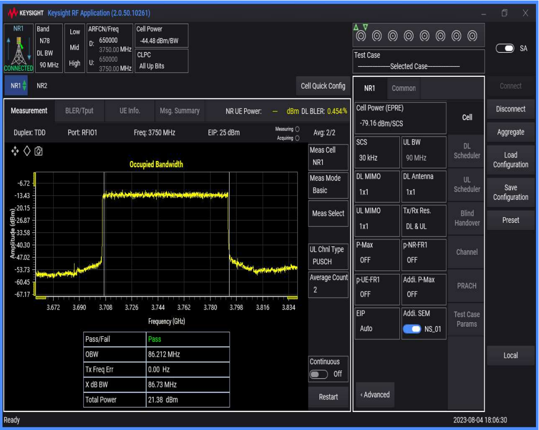
n78(3700-3800) SCS=30kHz DFT_QAM16 BW=100MHz Channel=650000 RB=270@0
