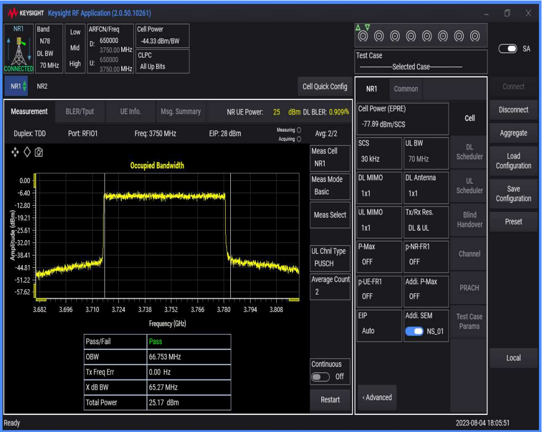
n78(3700-3800) SCS=30kHz DFT_QAM64 BW=80MHz Channel=650000 RB=216@0
