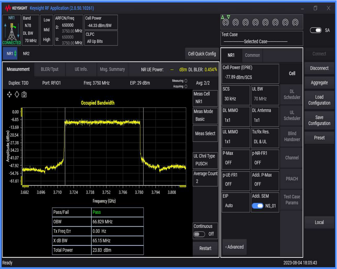
n78(3700-3800) SCS=30kHz DFT_BPSK BW=80MHz Channel=650000 RB=216@0
