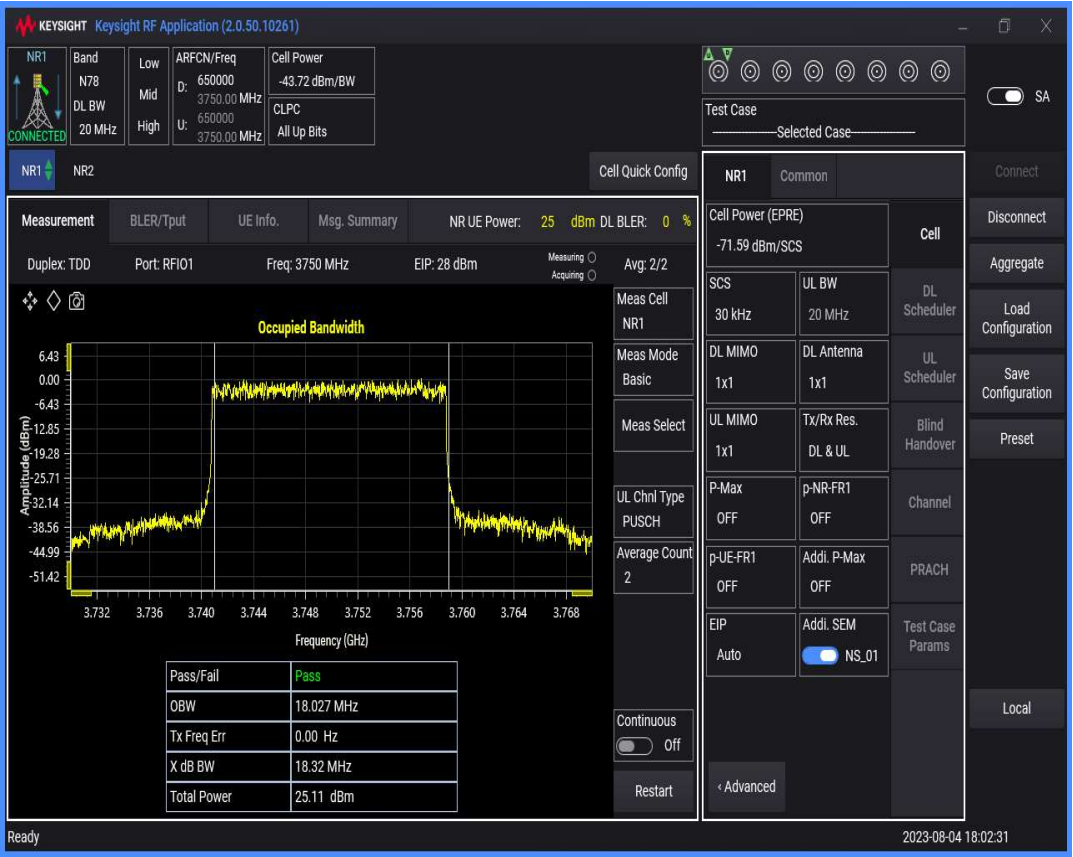
n78(3700-3800) SCS=30kHz DFT_QAM16 BW=30MHz Channel=650000 RB=75@0
