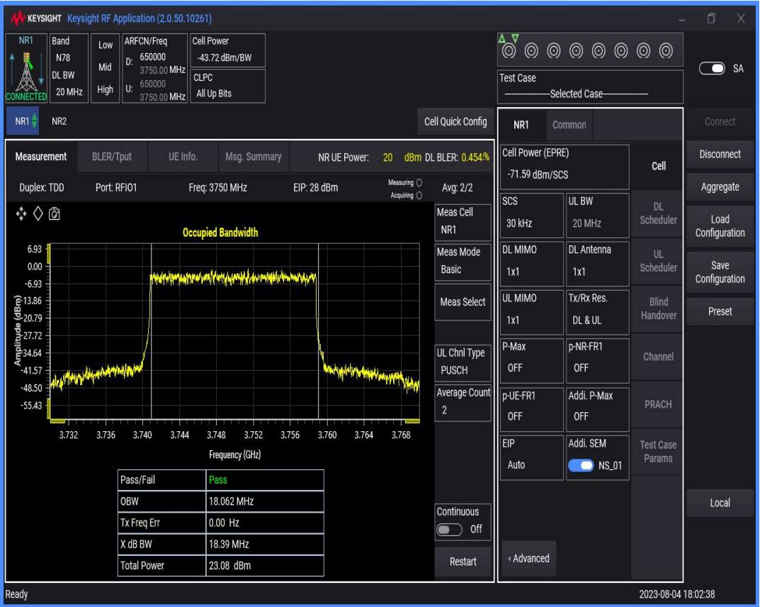
n78(3700-3800) SCS=30kHz DFT_QAM256 BW=30MHz Channel=650000 RB=75@0
