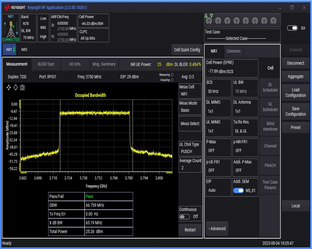
n78(3700-3800) SCS=30kHz DFT_QPSK BW=80MHz Channel=650000 RB=216@0
