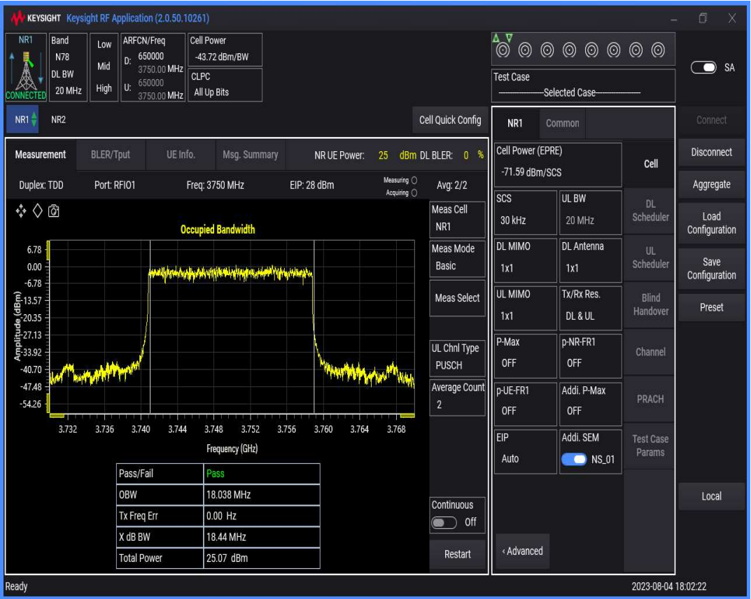
n78(3700-3800) SCS=30kHz DFT_BPSK BW=30MHz Channel=650000 RB=75@0
