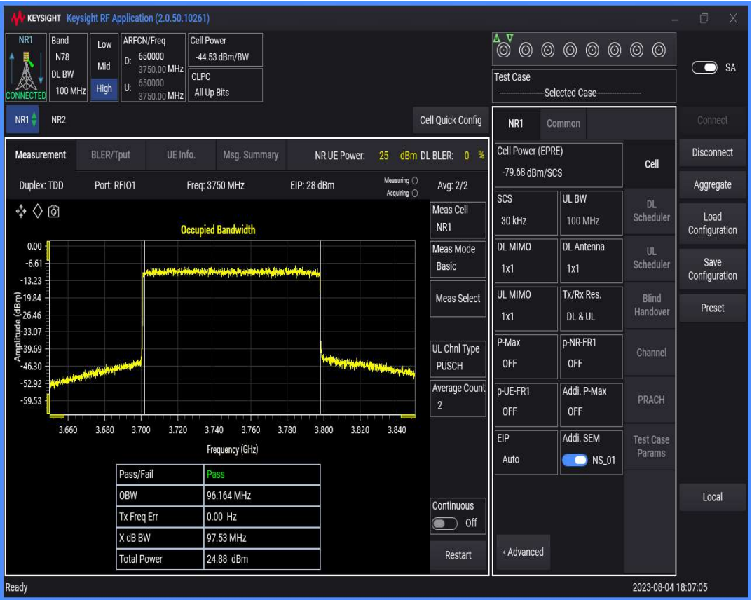
n78(3700-3800) SCS=30kHz DFT_QAM64 BW=10MHz Channel=650000 RB=24@0
