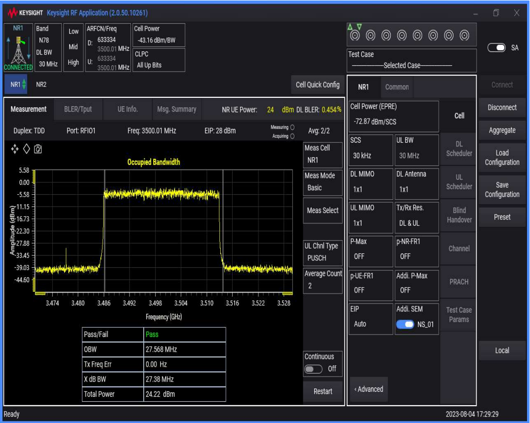
n78(3450-3550) SCS=30kHz DFT_QAM64 BW=40MHz Channel=633334 RB=100@0
