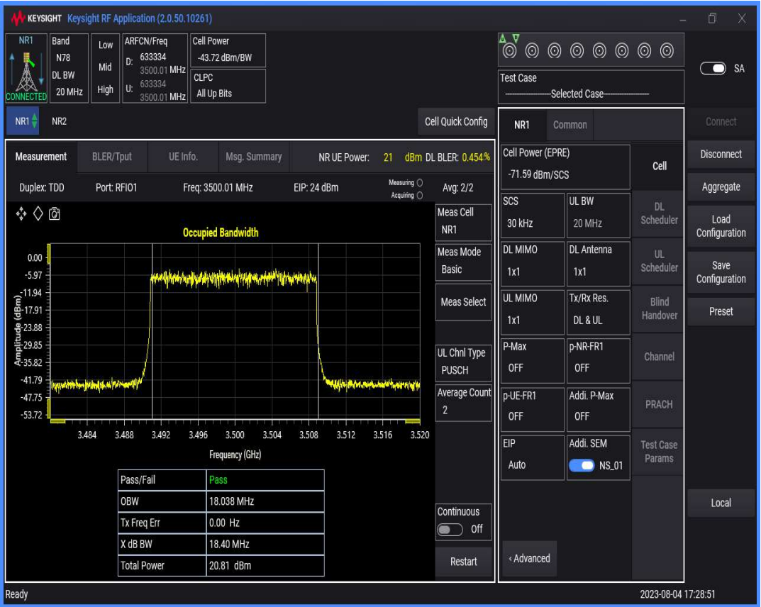
n78(3450-3550) SCS=30kHz DFT_BPSK BW=30MHz Channel=633334 RB=75@0
