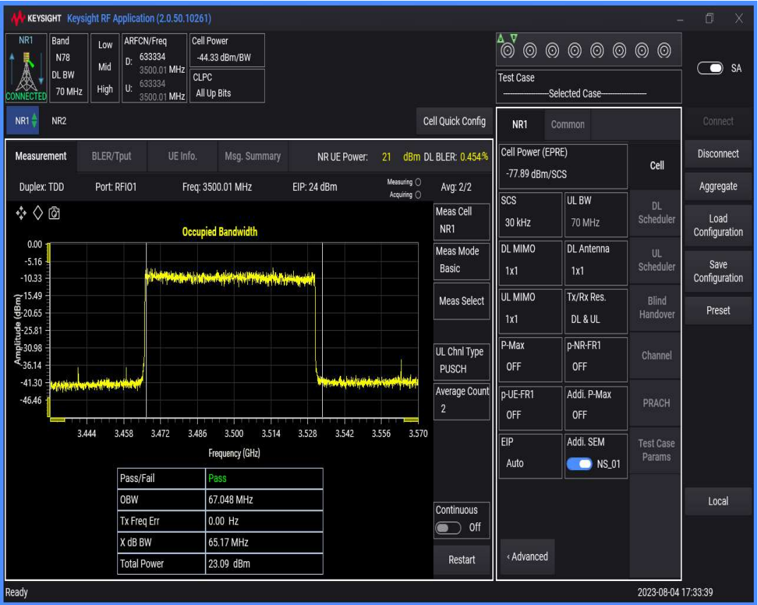
n78(3450-3550) SCS=30kHz DFT_QAM16 BW=80MHz Channel=633334 RB=216@0
