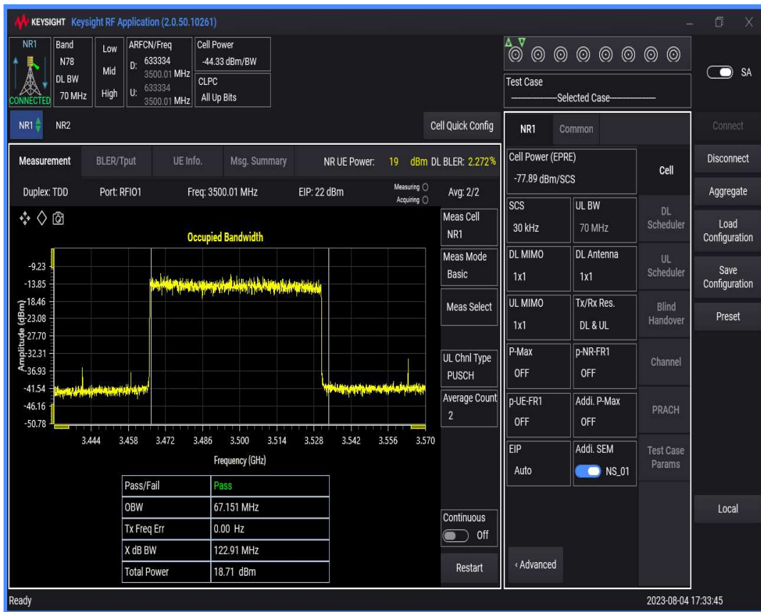
n78(3450-3550) SCS=30kHz DFT_QAM256 BW=80MHz Channel=633334 RB=216@0
