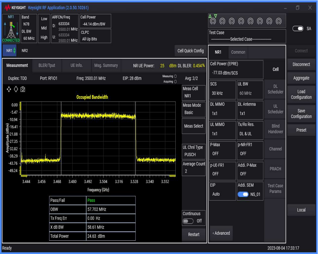
n78(3450-3550) SCS=30kHz DFT_QAM16 BW=70MHz Channel=633334 RB=
