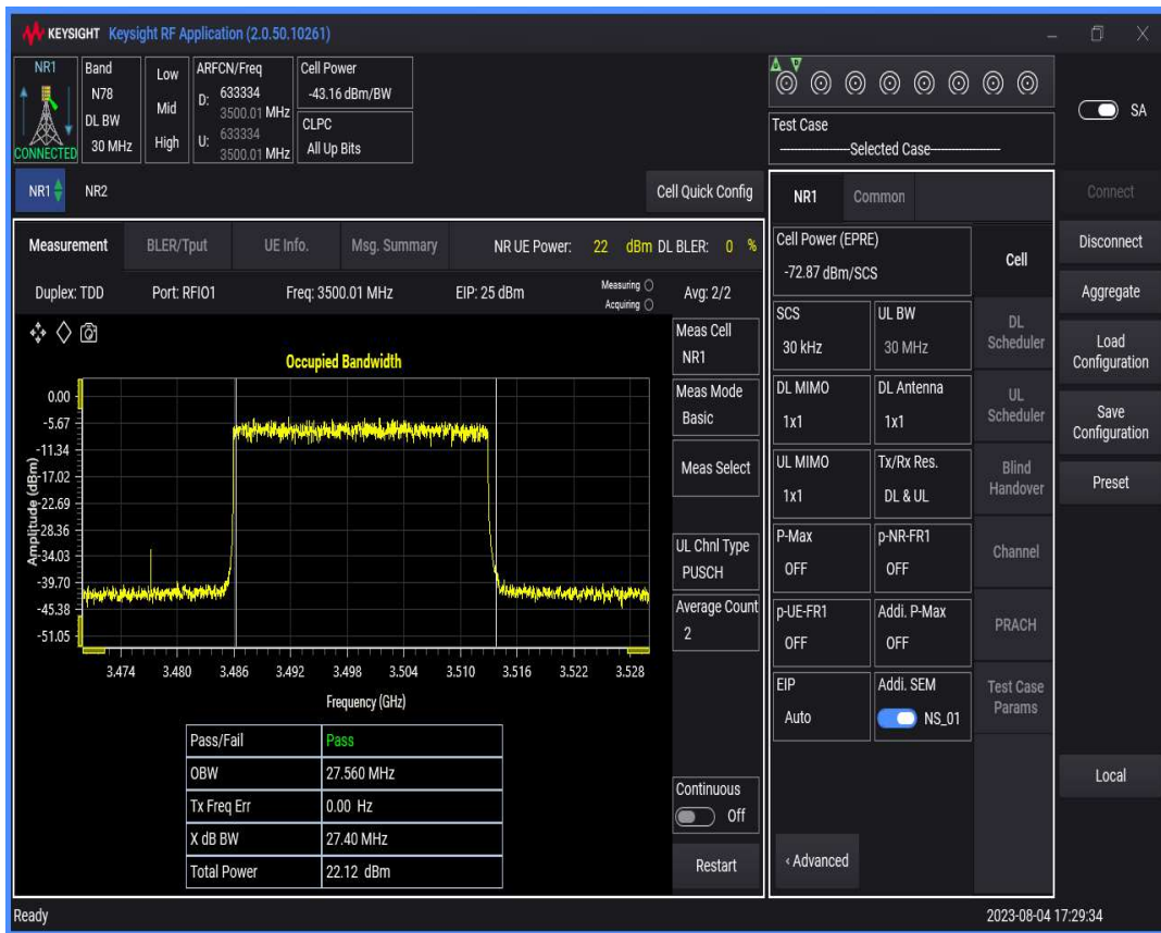
n78(3450-3550) SCS=30kHz DFT_QAM256 BW=40MHz Channel=633334 RB=100@0
