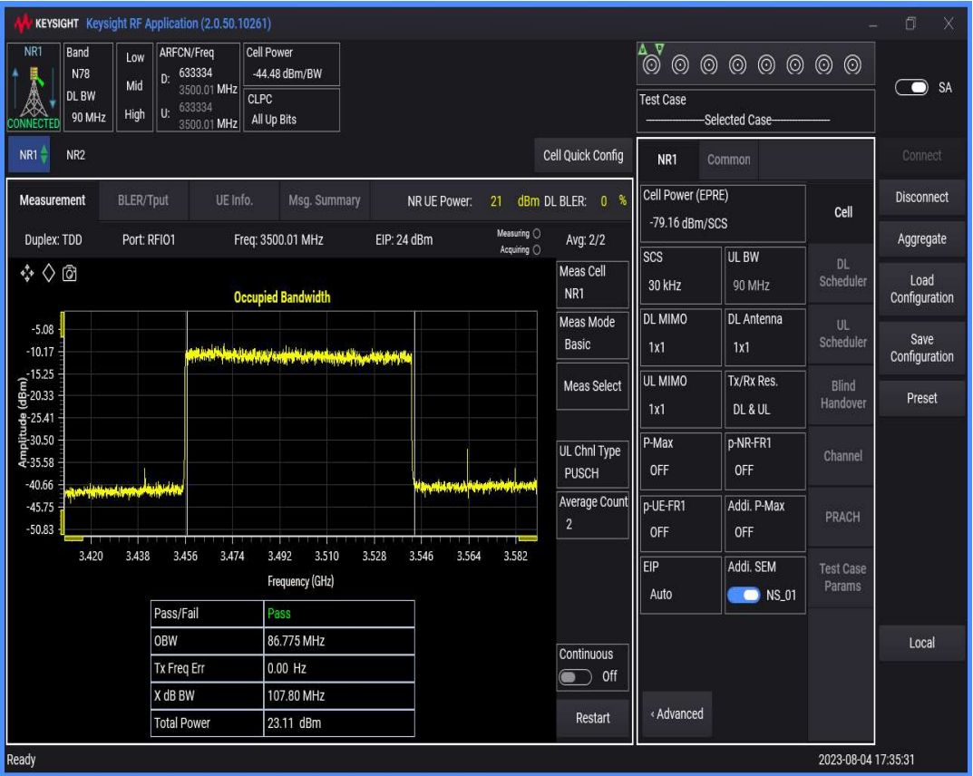
n78(3450-3550) SCS=30kHz DFT_QAM256 BW=100MHz Channel=633334 RB=270@0
