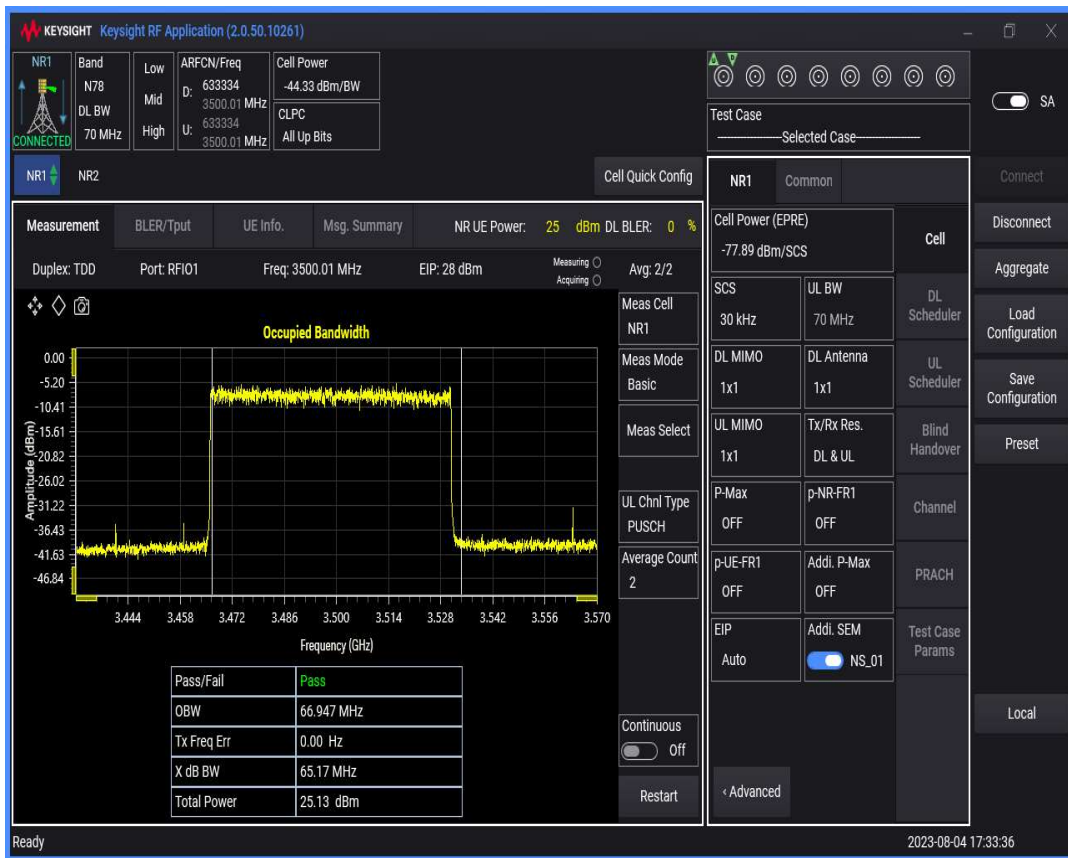
n78(3450-3550) SCS=30kHz DFT_QPSK BW=80MHz Channel=633334 RB=216@0
