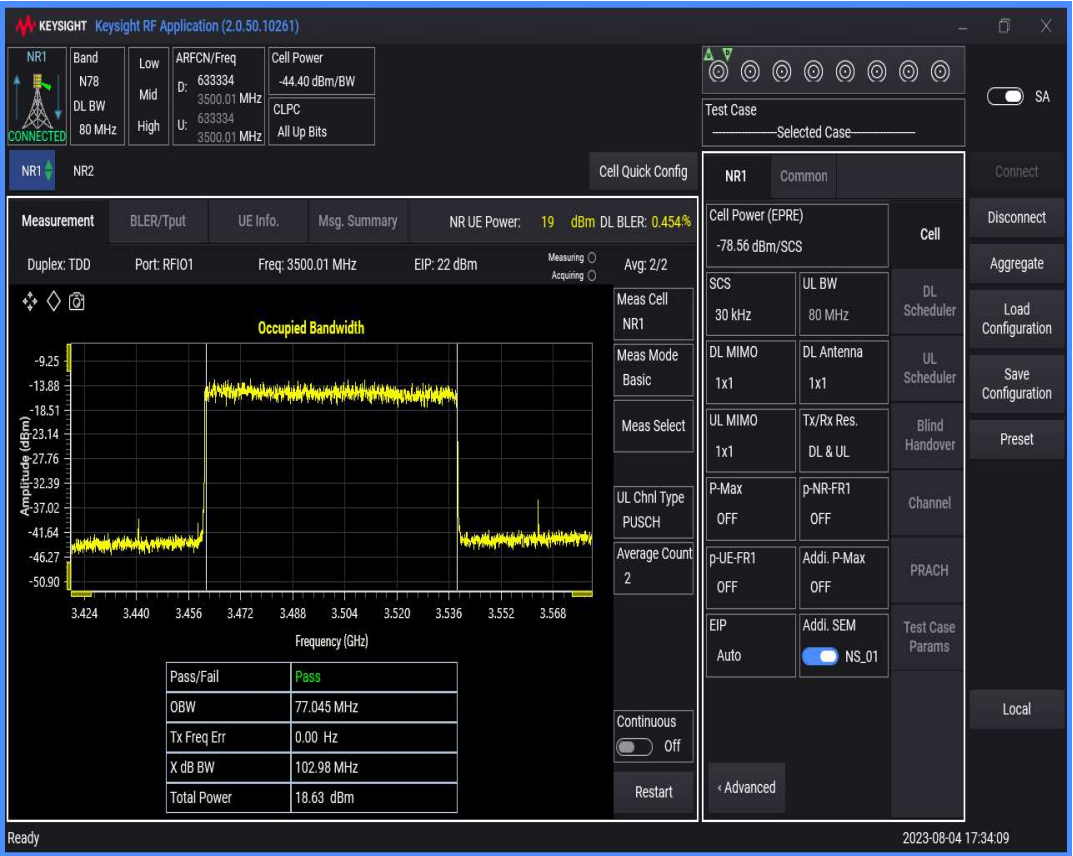
n78(3450-3550) SCS=30kHz DFT_QAM256 BW=90MHz Channel=633334 RB=240@0
