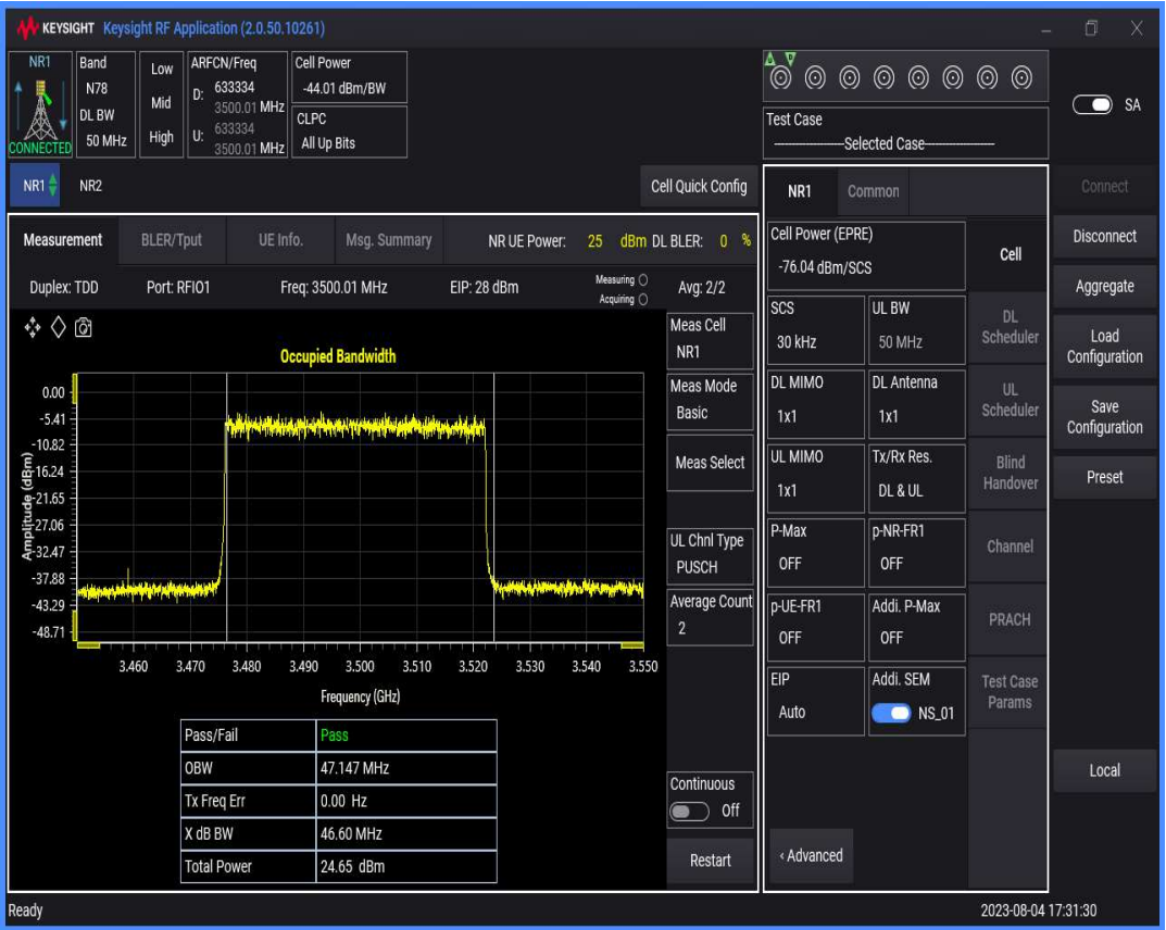
n78(3450-3550) SCS=30kHz DFT_QAM16 BW=60MHz Channel=633334 RB=162@0
