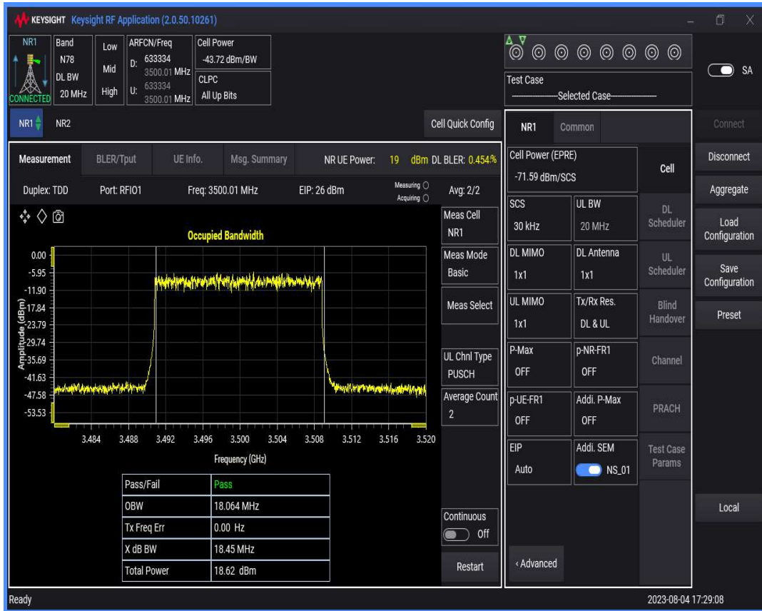
n78(3450-3550) SCS=30kHz DFT_QAM256 BW=30MHz Channel=633334 RB=75@0
