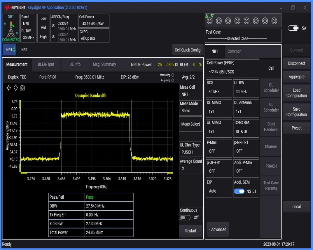
n78(3450-3550) SCS=30kHz DFT_BPSK BW=40MHz Channel=633334 RB=100@0
