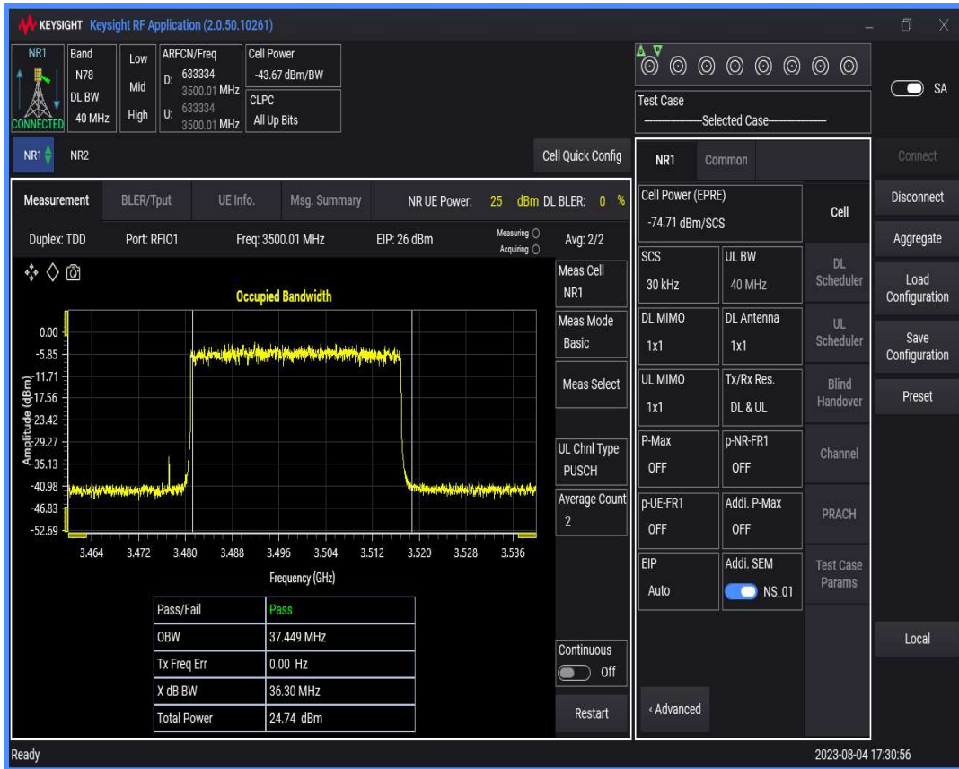
n78(3450-3550) SCS=30kHz DFT_BPSK BW=50MHz Channel=633334 RB=128@0
