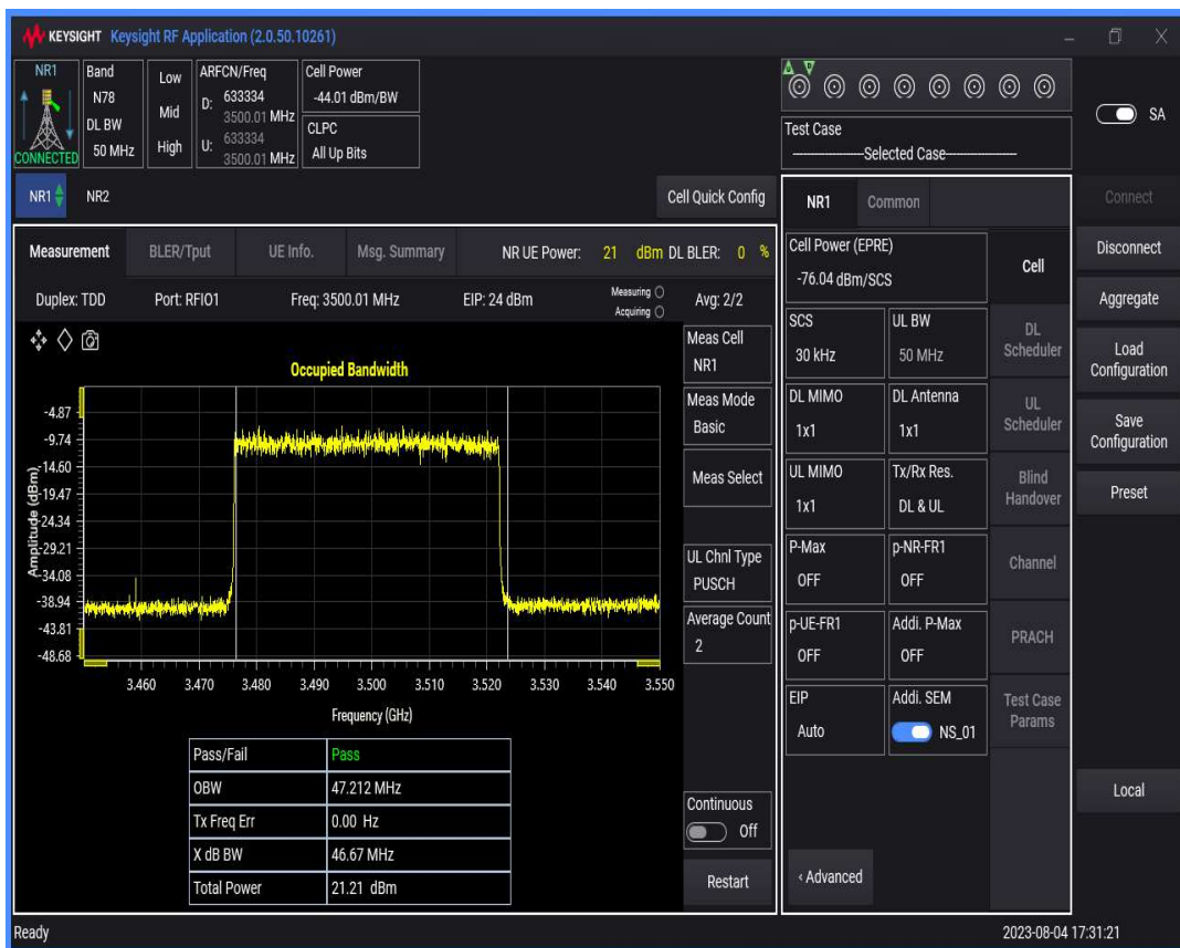
n78(3450-3550) SCS=30kHz DFT_BPSK BW=60MHz Channel=633334 RB=162@0
