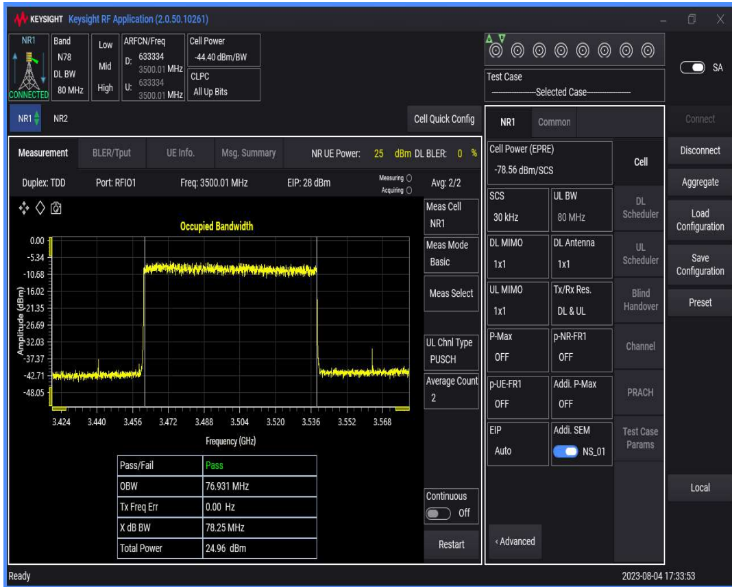
n78(3450-3550) SCS=30kHz DFT_BPSK BW=90MHz Channel=633334 RB=240@0
