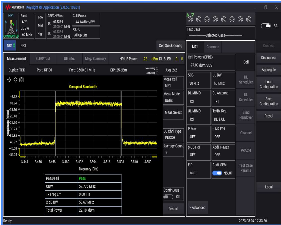
n78(3450-3550) SCS=30kHz DFT_QAM256 BW=70MHz Channel=633334 RB=
