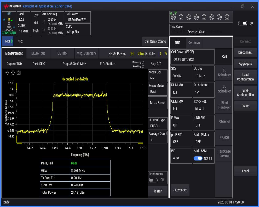
n78(3450-3550) SCS=30kHz DFT_QAM64 BW=15MHz Channel=633334 RB=36@0
