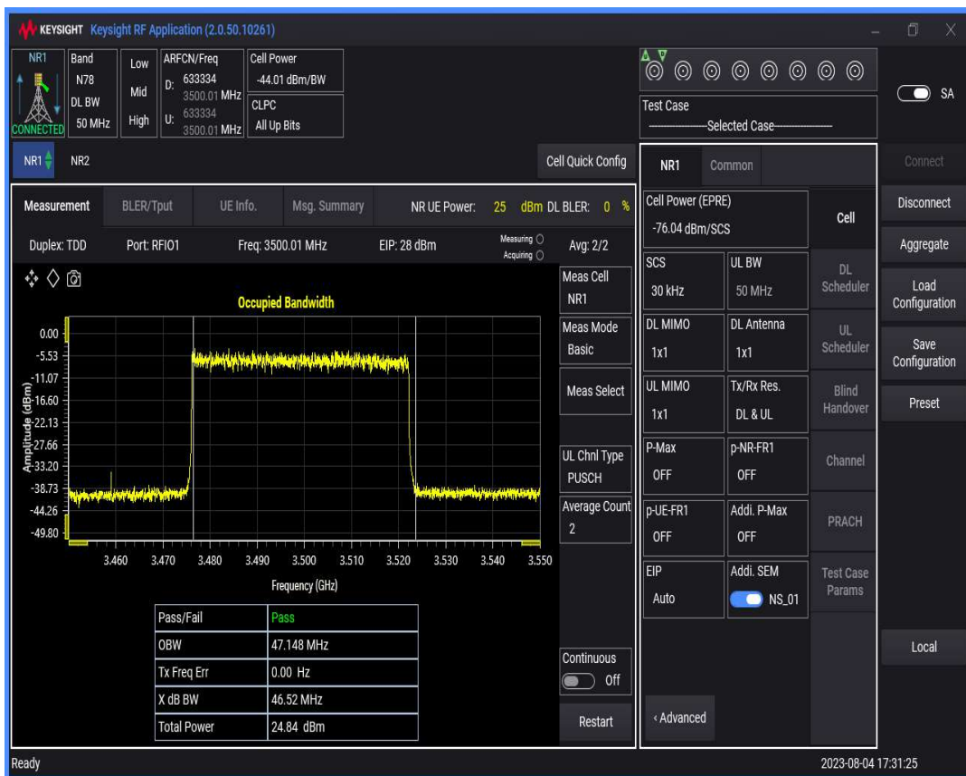
n78(3450-3550) SCS=30kHz DFT_QPSK BW=60MHz Channel=633334 RB=162@0
