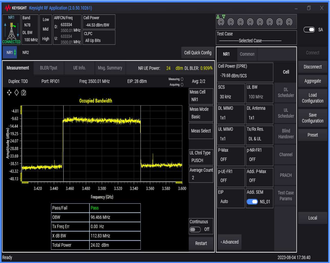
n78(3450-3550) SCS=30kHz DFT_QAM64 BW=10MHz Channel=633334 RB=24@0
