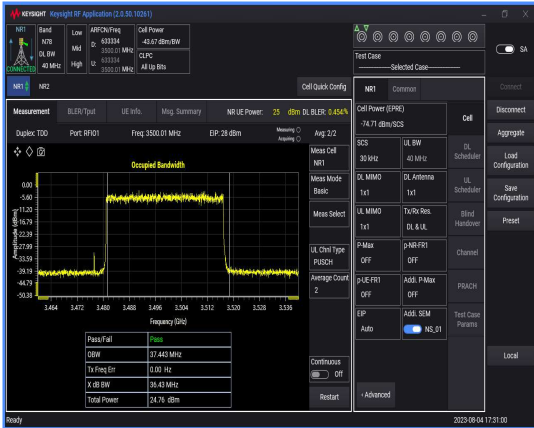
n78(3450-3550) SCS=30kHz DFT_QPSK BW=50MHz Channel=633334 RB=128@0
