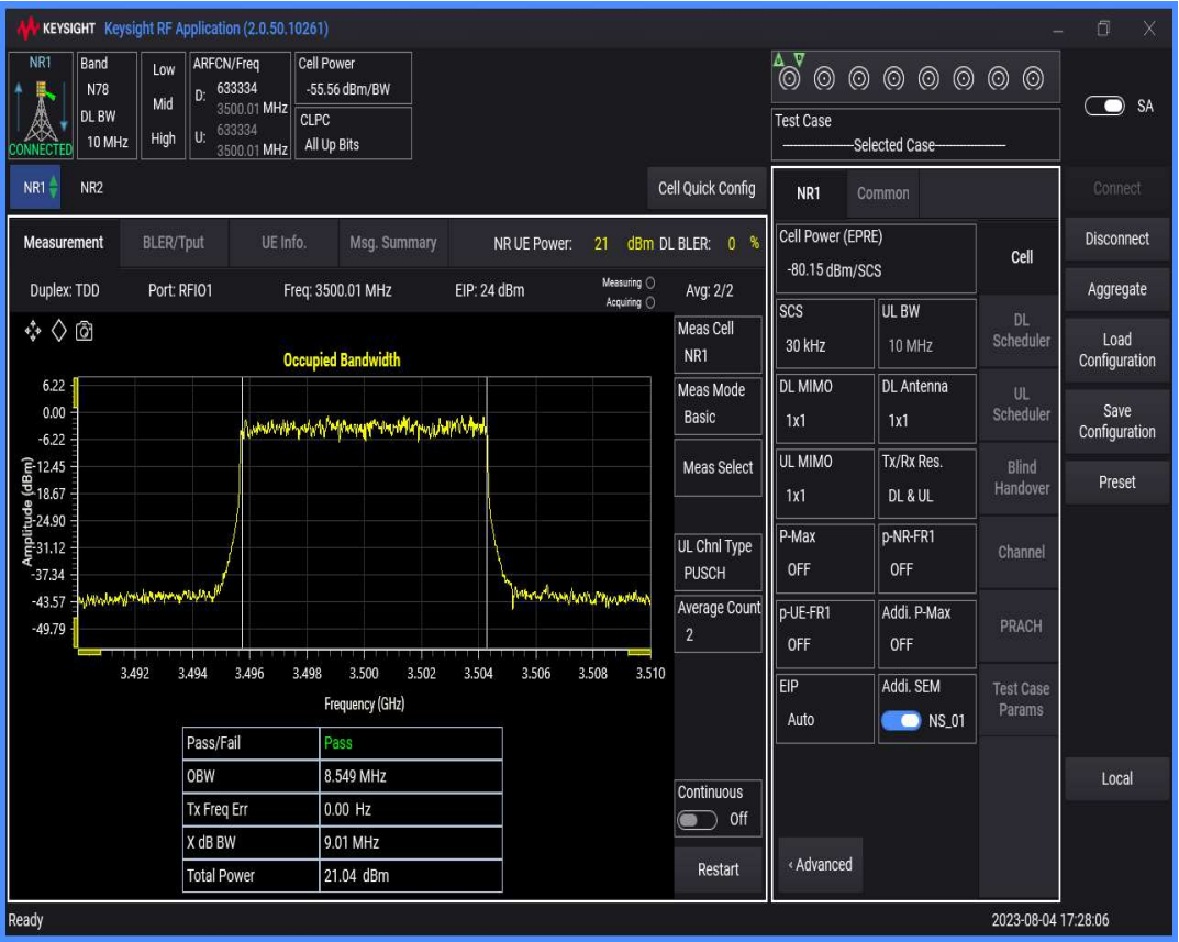
n78(3450-3550) SCS=30kHz DFT_QAM16 BW=15MHz Channel=633334 RB=36@0
