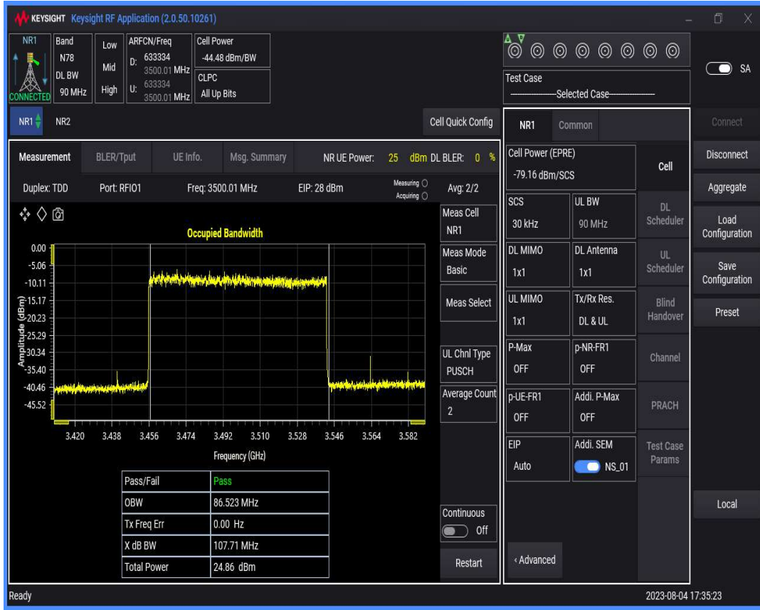
n78(3450-3550) SCS=30kHz DFT_QAM16 BW=100MHz Channel=633334 RB=270@0
