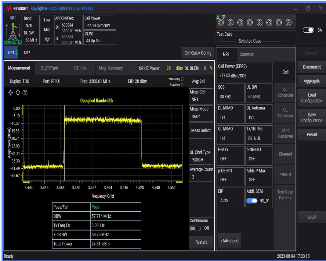
n78(3450-3550) SCS=30kHz DFT_QPSK BW=70MHz Channel=633334 RB=
