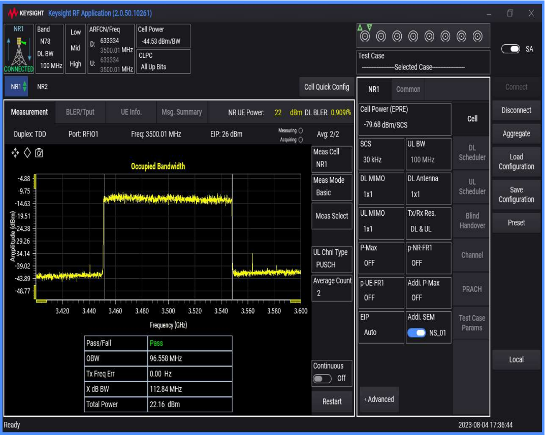
n78(3450-3550) SCS=30kHz DFT_QAM256 BW=10MHz Channel=633334 RB=24@0
