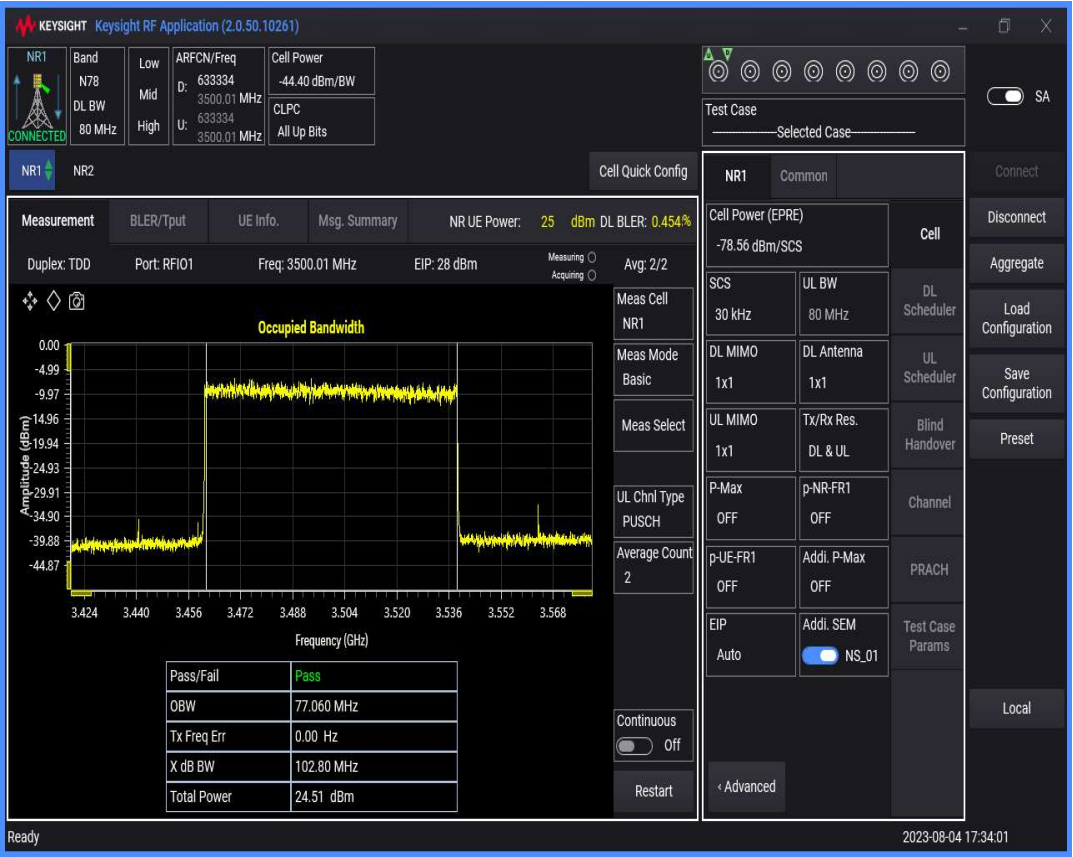
n78(3450-3550) SCS=30kHz DFT_QAM16 BW=90MHz Channel=633334 RB=240@0
