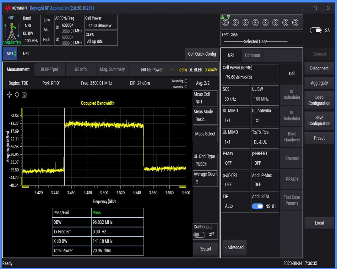
n78(3450-3550) SCS=30kHz DFT_QAM16 BW=10MHz Channel=633334 RB=24@0
