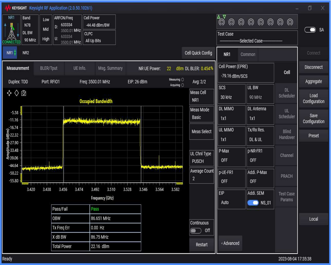
n78(3450-3550) SCS=30kHz DFT_QAM64 BW=100MHz Channel=633334 RB=270@0
