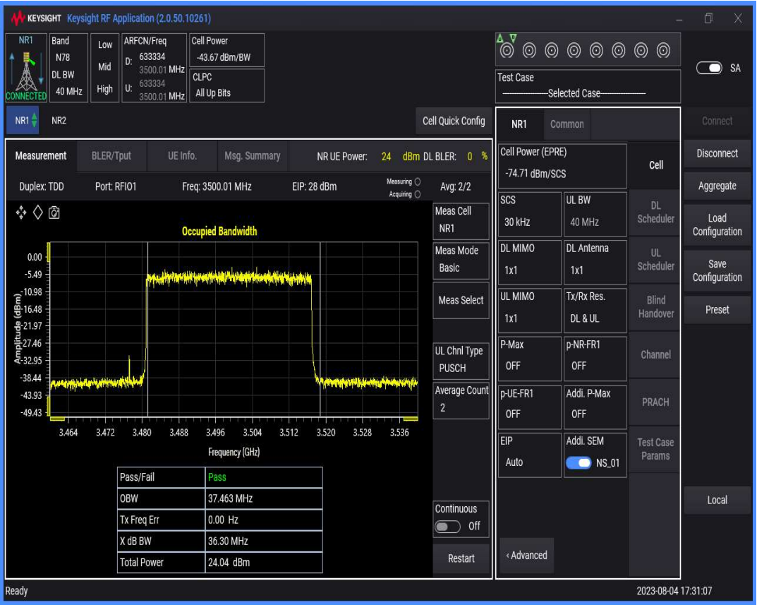
n78(3450-3550) SCS=30kHz DFT_QAM64 BW=50MHz Channel=633334 RB=128@0
