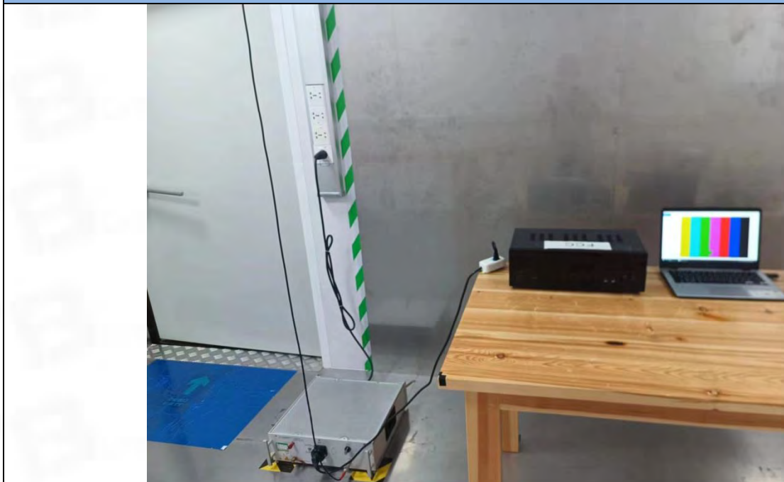
Conducted Emission at AC power line
