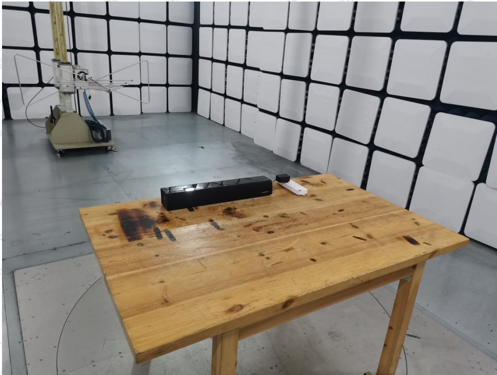
Photo of Radiation Emission Test
