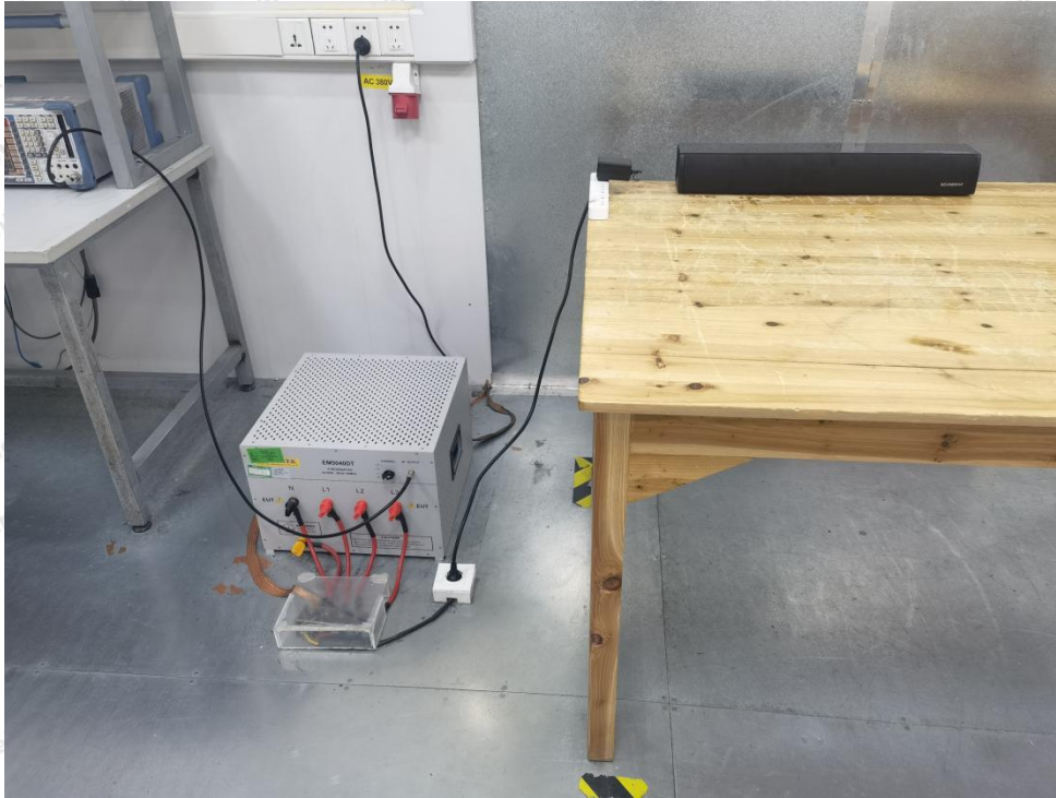
Photo of Conducted Emission Measurement
