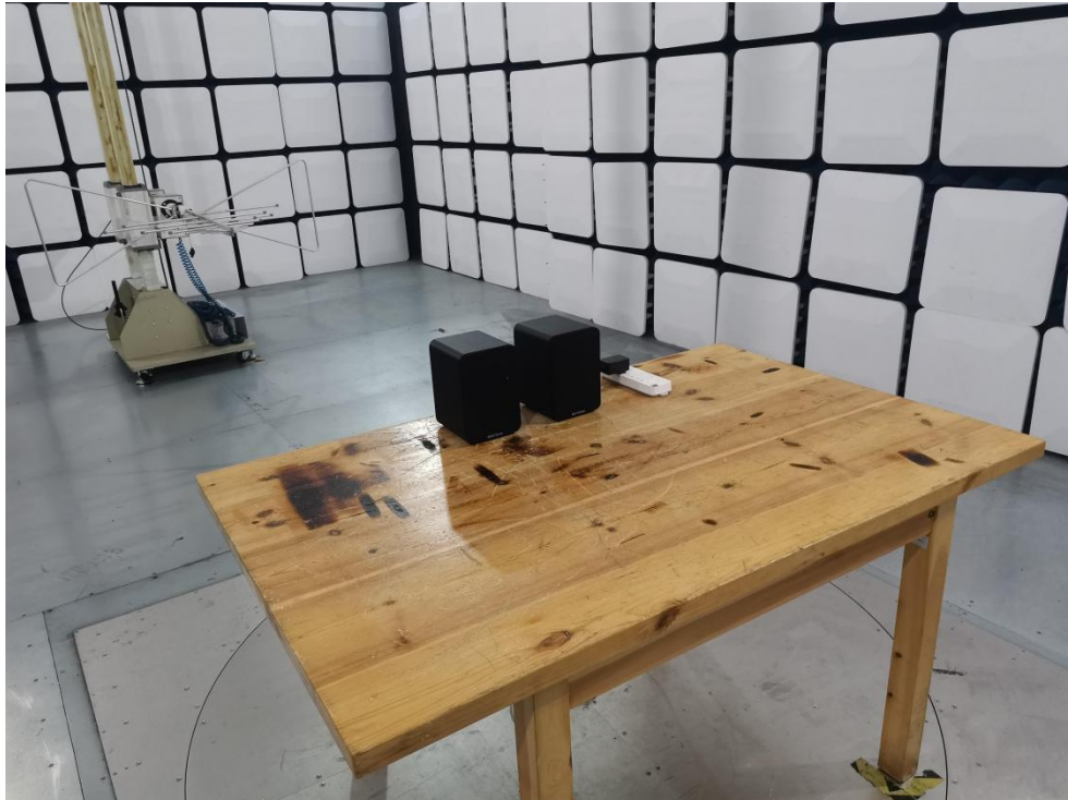
Photo of Radiation Emission Test
