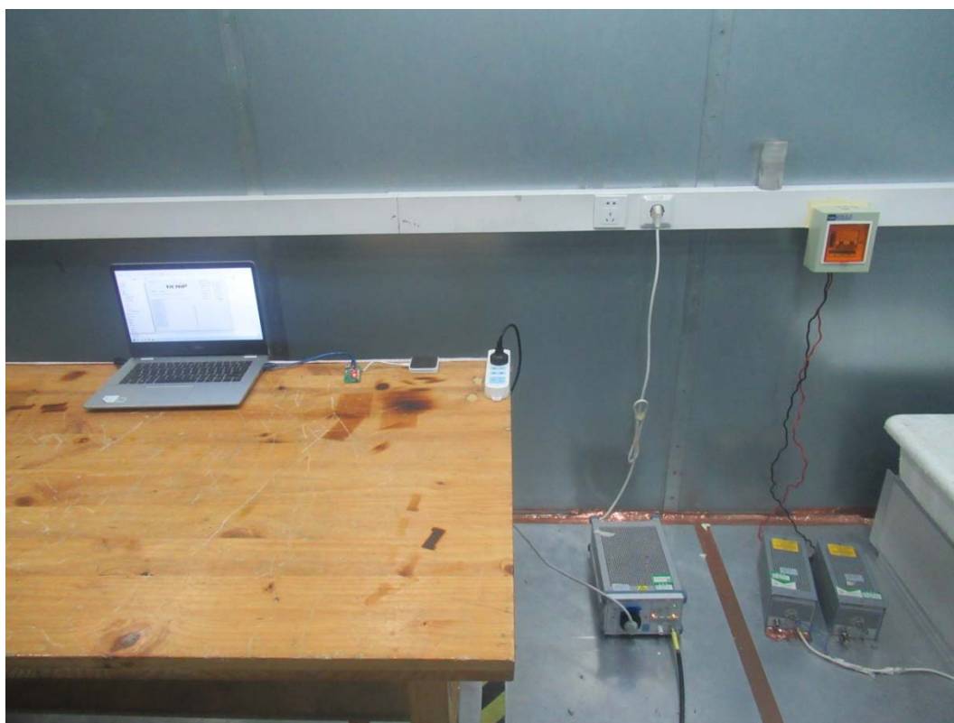
Picture 2: Conducted Emissions Test Setup
