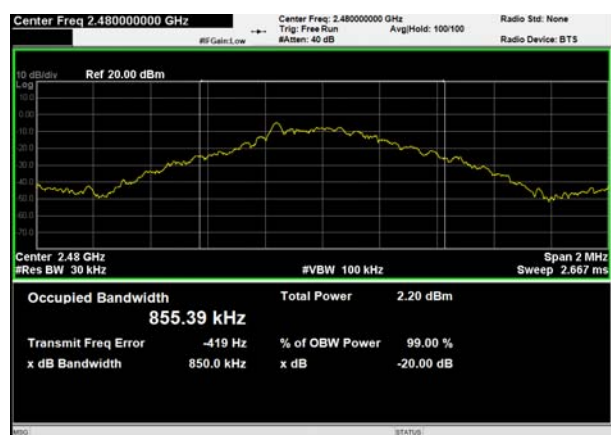
BT DH5 CH78, Carrier frequency (MHz): 2480
