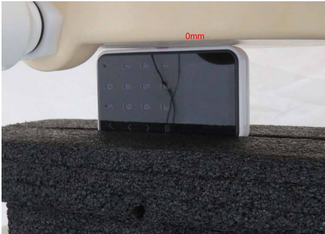
Picture 5: Left Edge, the distance from handset to the bottom of the Phantom is 0mm
