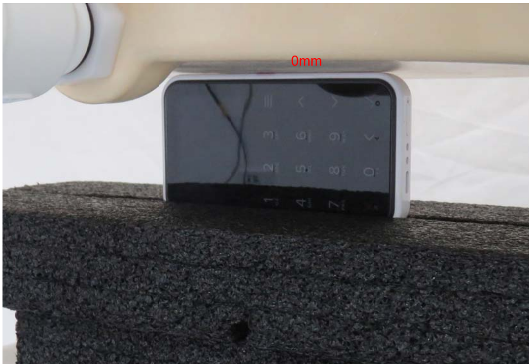
Picture 6: Right Edge, the distance from handset to the bottom of the Phantom is 0mm
