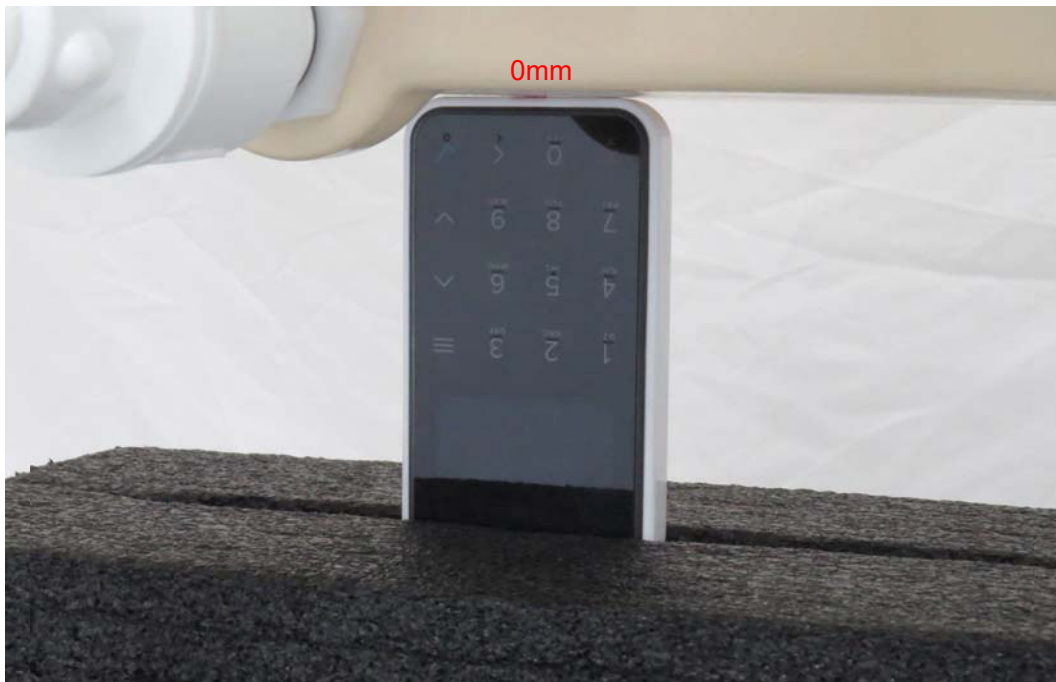
Picture 8: Bottom Edge, the distance from handset to the bottom of the Phantom is 0mm
