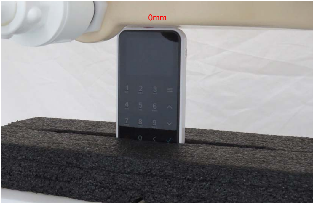
Picture 7: Top Edge, the distance from handset to the bottom of the Phantom is 0mm
