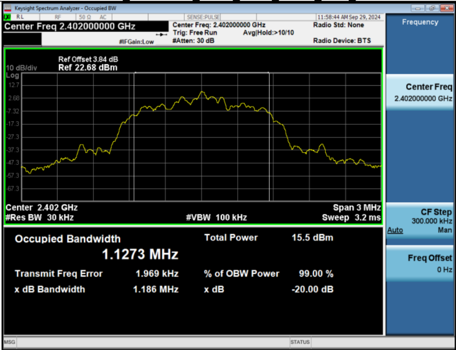
-20dB Bandwidth NVNT ANT1 2-DH1 2402 00
