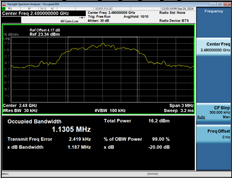
-20dB Bandwidth NVNT ANT1 2-DH1 2480 00
