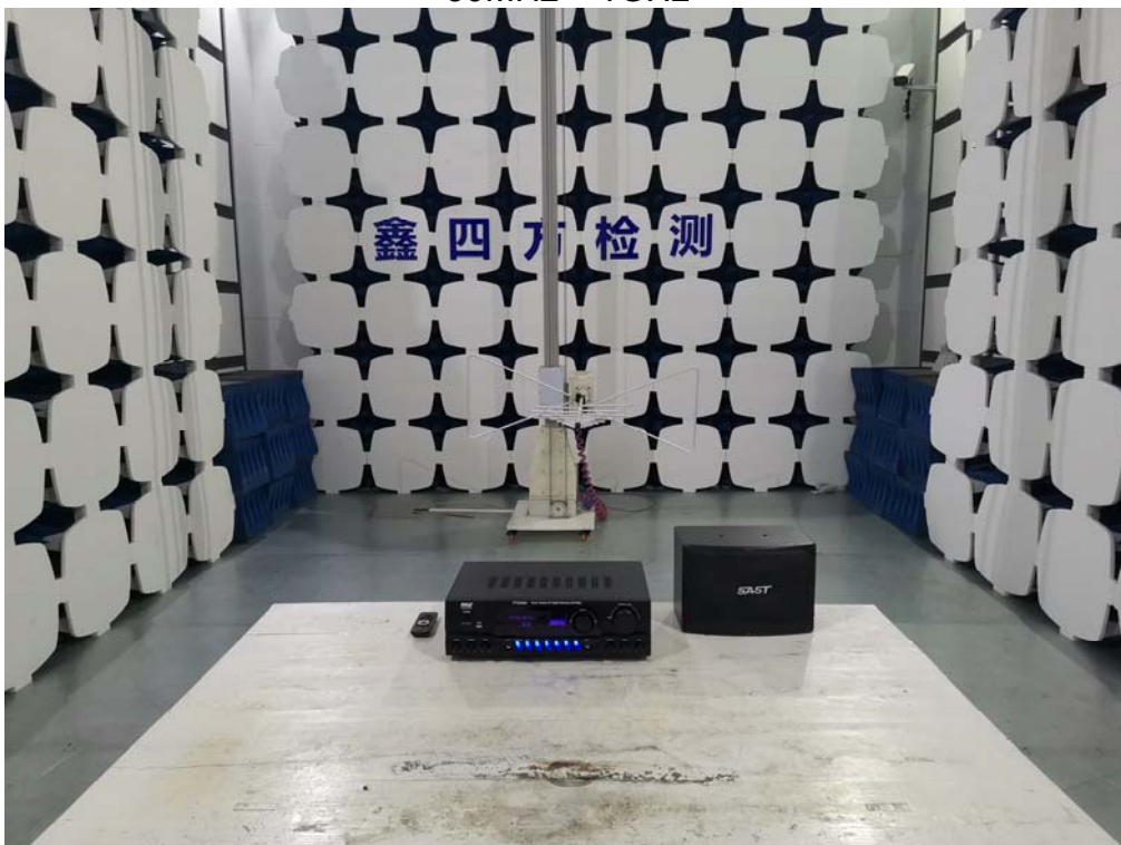
Photos of radiated emission test 30MHz – 1GHz
