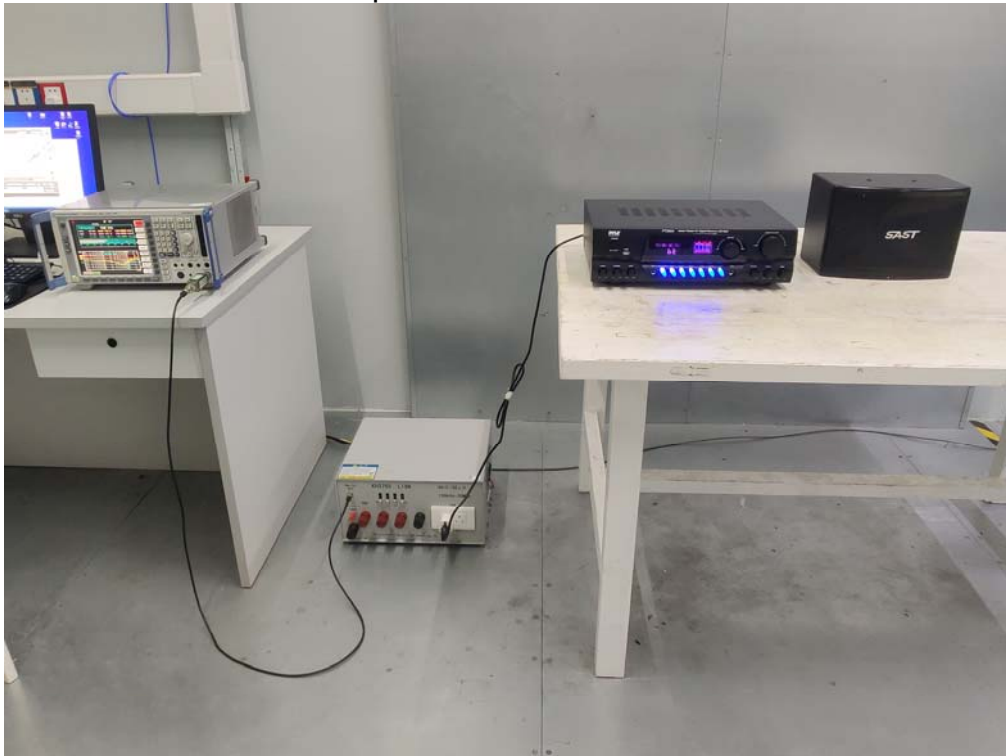
Photos of radiated emission test 30MHz – 1GHz
