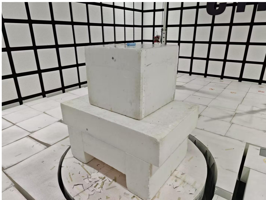
Radiated spurious emission Test Setup-3(Above 1GHz)
