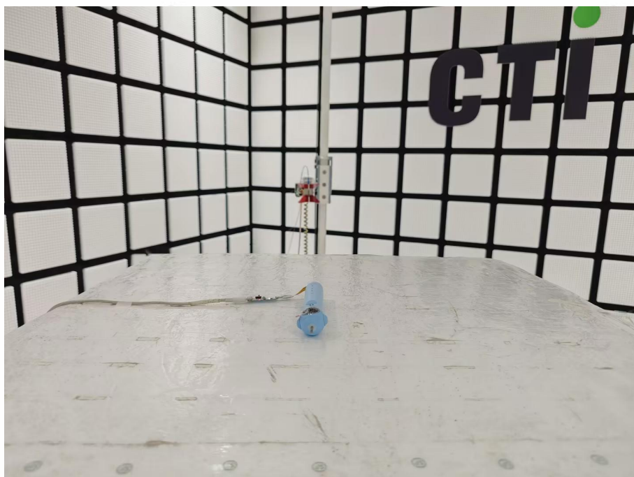
Radiated spurious emission Test Setup-4(Above 1GHz)
