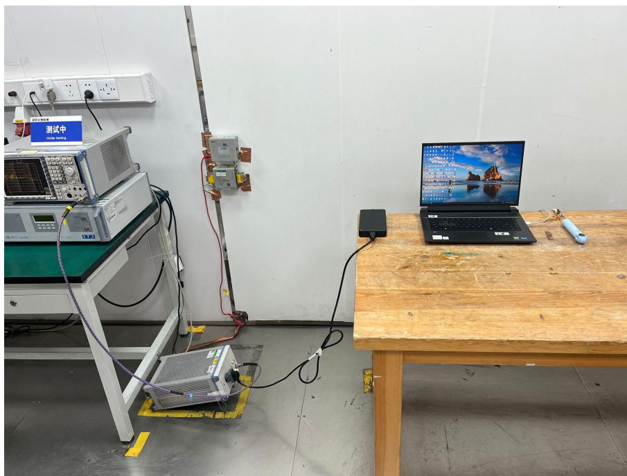
Conducted Emissions Test Setup
