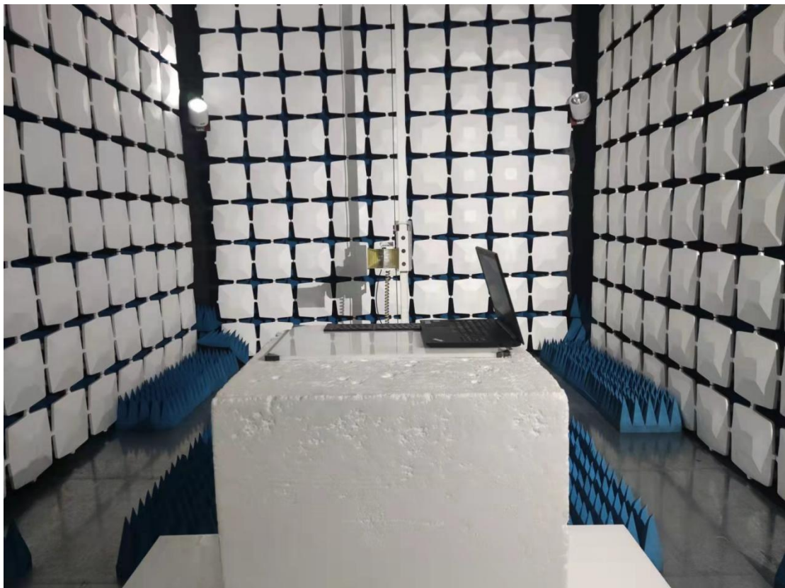
Above 1GHz for radiated emission test setup
