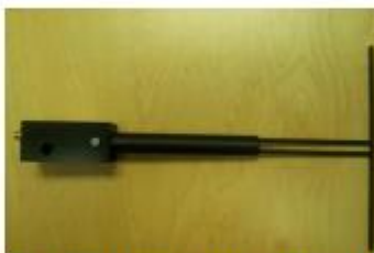
Figure 1 – MVG COMOSAR Validation Dipole
