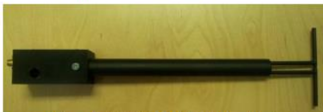
Figure 1 – MVG COMOSAR Validation Dipole
