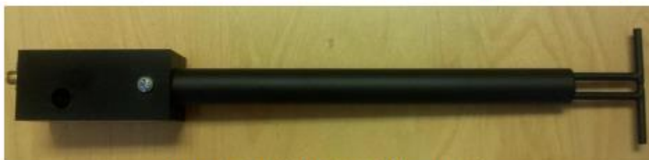
Figure 1 – MVG COMOSAR Validation Dipole
