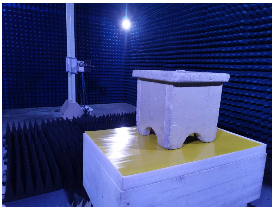
Photo of Radiated Emission Measurement (Above 1GHz)
