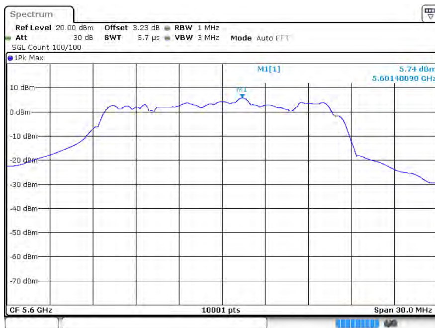
PSD ax20 5600MHz Ant2
