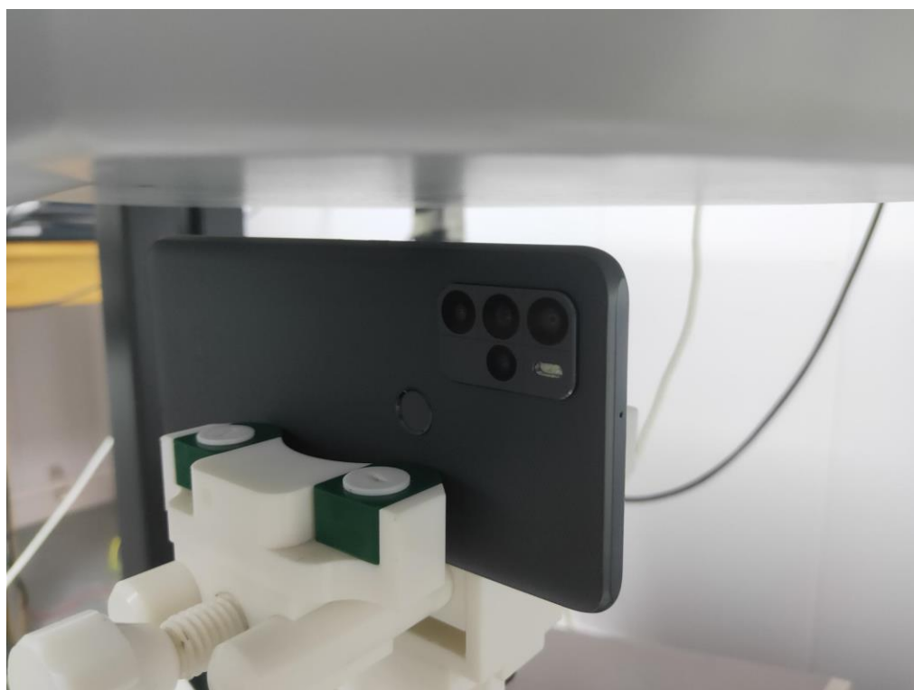
10mm body-worn Right Side Setup Photo (hotspot)
