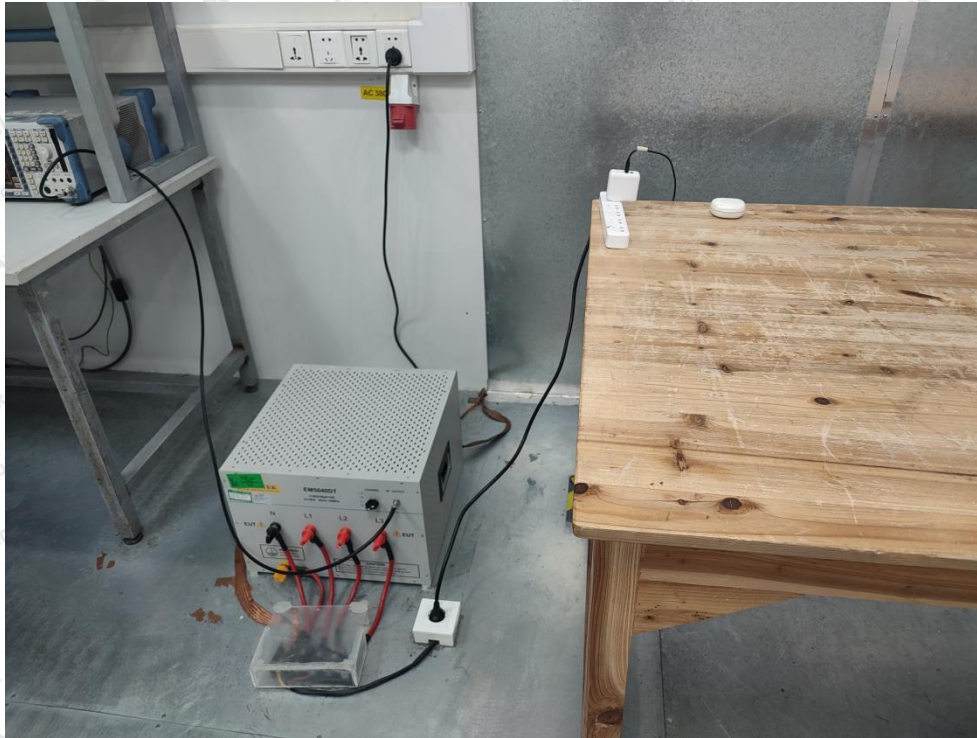
Photo of Conducted Emission Measurement
