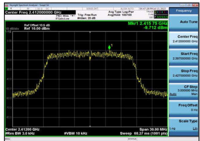
Power spectral density-802.11g ,2462MHz,Ant0
