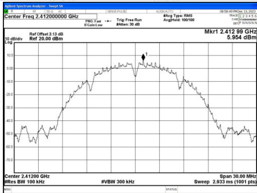
Band Edge NVNT b 2412MHz Ant1 Emission
