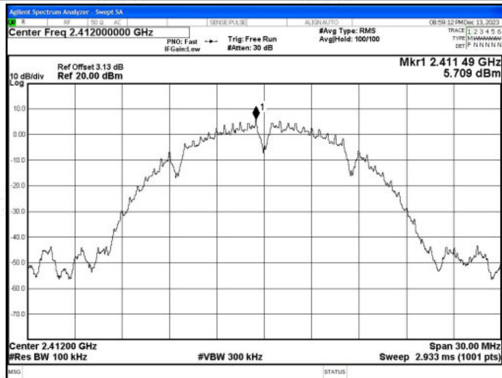
Tx. Spurious NVNT b 2412MHz Ant1 Emission
