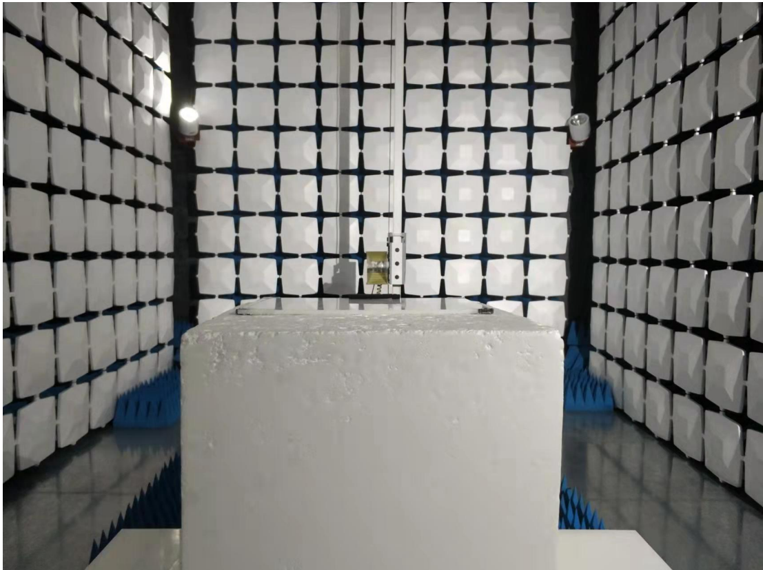
Above 1GHz for radiated emission test setup
